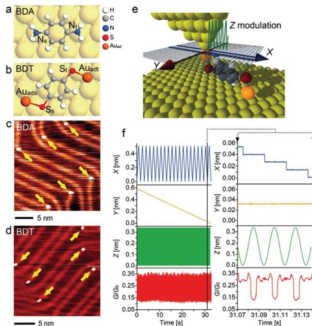
**Fig. 1** Measurement setup. (a, b) Schematics of the molecular structures of BDA and BDT deposited on a Au(111) surface, respectively. (c, d) STM images of BDA and BDT molecules on a Au (111) surface, respectively. (e) Schematic of the 3D dynamic probe method. (f) Schematic of the measurement scheme.
