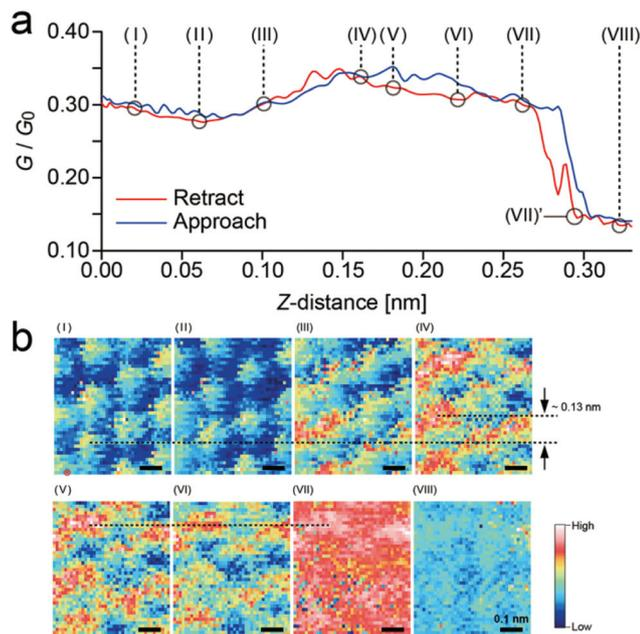
**Fig. 4** Data obtained for BDT. (a) Typical conductance curves of a BDT molecule obtained by the retract and approach motion. (b) XY conductance map corresponding to the Z-positions (I) to (VIII) in (a).
