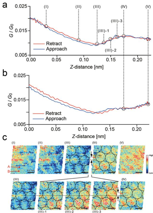
Fig. 3 Data obtained for BDA. (a, b) Two typical conductance curves of a BDA molecule obtained by the retract and approach motion at positions A and B in (c) (i). (c) *XY* conductance maps corresponding to the *Z*-positions (I) to (V) in (a).
