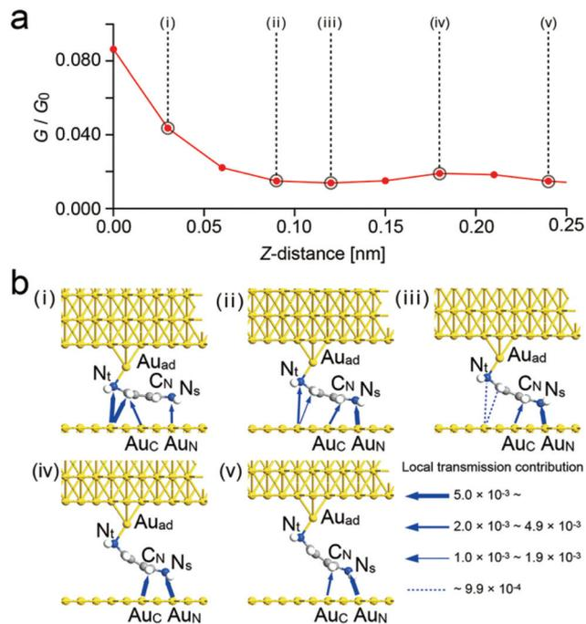
**Fig. 5** Simulated conductance curve obtained for BDA. (a) Simulated conductance curve corresponding to the change from (i) to (v) in Fig. 3a. (b) Schematics of conformational structures and local transmission contributions for (i) to (v) in (a). Local transmission contributions are proportional to the thickness of the arrows.
