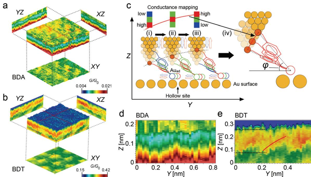
**Fig. 2** 3D plot and the analysis method. (a, b) 3D plots obtained for BDA and BDT molecules, respectively. (c) Schematic diagram to determine the adsorption angle.  $\varphi$  represents the angle between the molecule and the substrate considering the direction of the molecule (see Fig. S1† for details). (d, e) YZ cross sections for the cases of BDA and BDT, respectively.
