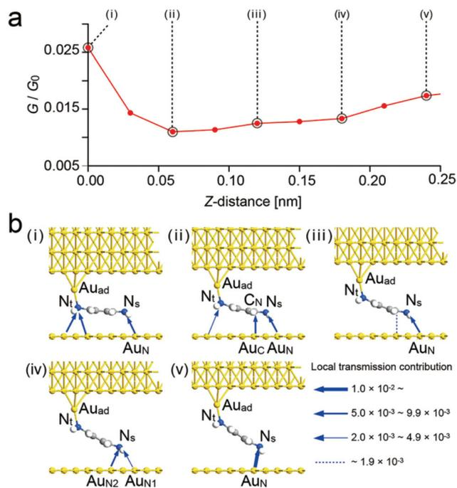
**Fig. 6** Simulated conductance curve obtained for BDA. (a) Simulated conductance curve corresponding to the change from (i) to (v) in Fig. 4b. (b) Schematics of conformational structures and local transmission contributions for (i) to (v) in (a). Local transmission contributions are proportional to the thickness of the arrows.
