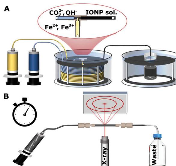
**Fig. 1** (A) Schematic of the set-up for nanoparticle synthesis showing the syringe pumps used to feed reactants to a T-mixer, pre-heated water bath, and aging bath. (B) Schematic of the synchrotron X-ray diffraction set-up showing the solution injected into a quartz capillary for analysis.
