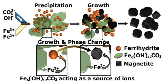
Fig. 6 Schematic of growth mechanism showing the initial precipitation of iron hydroxide carbonate [ $\text{Fe}_6(\text{OH})_{12}\text{CO}_3$ ] and ferrihydrite and the growth of ferrihydrite via the re-dissolution of iron hydroxide carbonate to form the magnetite phase.
