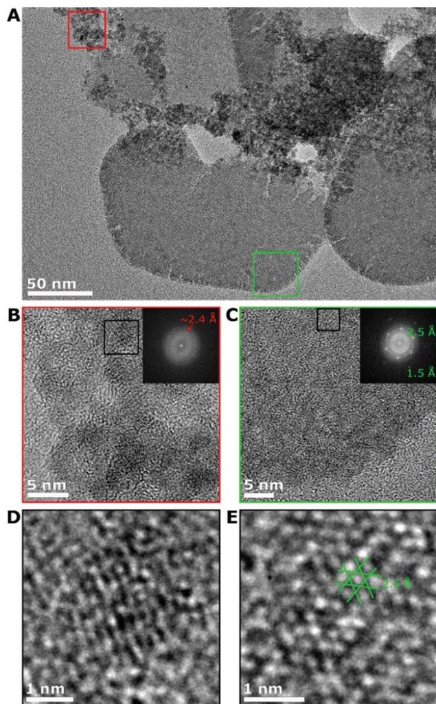
**Fig. 3** (A) Aberration corrected TEM image of the sample taken at 2 min of an area with particles and plates present. High resolution images taken of (B) the particles from the red box, and (C) the plate from the green box. Both images have the Fourier transforms of the image as an inset with the spacing of the spots/rings indicated on the inset. (D) and (E) are zoomed in on the areas in the black boxes of (B) and (C) showing the crystallinity of the structures.
