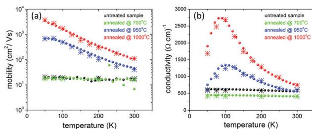
**Fig. 4** Temperature dependence of (a) the mobility and (b) the conductivity for the four samples. Dots are for the experiment and stars are for the calculations.
