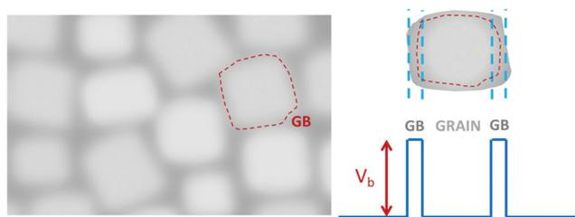
**Fig. 1** Schematic of the nanocrystalline structure. Bulk-like grains (light shaded areas) are separated by grain boundaries (GBs) (red dashed line). Charged defects around GBs (dark shaded areas) form potential barriers of height  $V_b$  for carriers.
