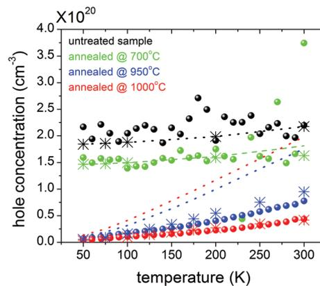
**Fig. 2** Temperature dependence of the hole concentration for samples: A (untreated), B (annealed at 700 °C), C (annealed at 950 °C) and D (annealed at 1000 °C). The colors for symbols and lines correspond to the samples as indicated in the legend. The mobile hole concentration is shown in dots (experiment) and in stars (calculations). The dotted lines are for the calculated hole concentration within the grain.
