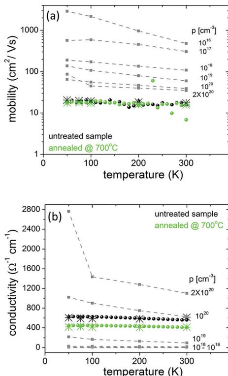
**Fig. 3** Temperature dependence of (a) the mobility and (b) the conductivity in the low- $T_a$  regime (samples A and B). The dots are for experimental data and the stars are for theoretical calculations. The squares are for the calculated  $T$ -dependence of the mobility and the conductivity of bulk Si in a wide hole concentration range shown for reference. The dashed lines are a guide to the eye.
