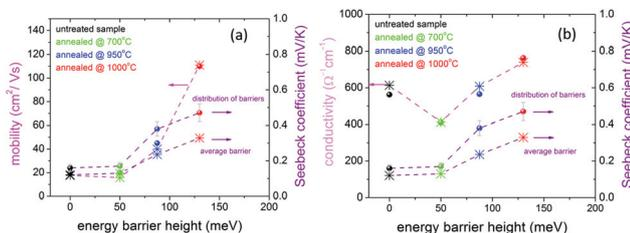
**Fig. 5** Simultaneous increase of the transport properties for high- $T_a$ . The mobility (left y-axis of (a)), the conductivity (left y-axis of (b)) and the Seebeck coefficient (right y-axes) at 300 K. Dots are for measurements and stars are for calculations. The dashed lines are a guide to the eye. The average energy barrier height for each sample was estimated by the  $T$ -dependences of the mobility and conductivity (Fig. 4).
