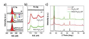
Fig. 5 XPS (a) C 1s and (b) Fe 2p spectrum of bare GF,  $Fe_2O_3$ -GF and RGO- $Fe_2O_3$ -GF composites; (c) XRD patterns of bare GF,  $Fe_2O_3$ -GF and RGO- $Fe_2O_3$ -GF composites.
