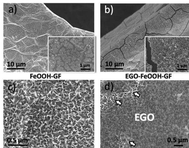
**Fig. 3** (a, b) SEM image of CVD–GF with low and high loading amounts of FeOOH: (a) 0.10 mg cm<sup>-2</sup>, (b) 0.39 mg cm<sup>-2</sup>. The insets show higher magnification of the surface. (c) FeOOH nano-walls grown on GF with a moderate loading (0.15 mg cm<sup>-2</sup>) showing a uniform nanowall morphology. (d) The same nano-walls of (c), coated with EGO. Brighter areas (shown by white arrows) indicate holes in the EGO coating.
