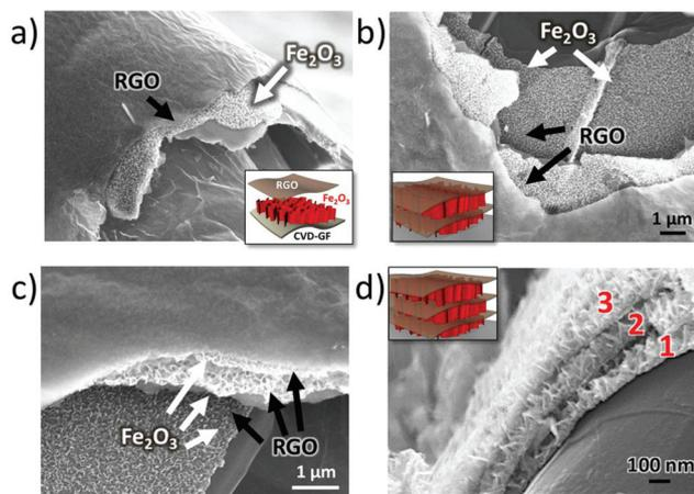
**Fig. 4** SEM images of GF coated with an increasing number of  $\text{Fe}_2\text{O}_3$  and RGO layers; (a) single RGO- $\text{Fe}_2\text{O}_3$  coating; (b) double (RGO- $\text{Fe}_2\text{O}_3$ )<sub>2</sub> coating; (c, d) triple (RGO- $\text{Fe}_2\text{O}_3$ )<sub>3</sub> coating. Red numbers in (d) indicate the well-separated different  $\text{Fe}_2\text{O}_3$  layers formed by vertical nanowalls. Insets show the schematic representation of the different layers in the sandwich structure.
