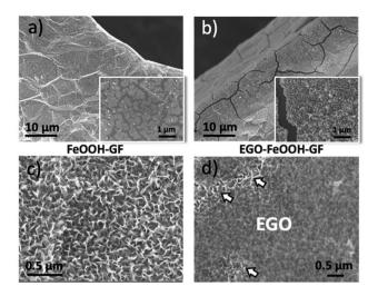
Fig. 3 (a, b) SEM image of CVD-GF with low and high loading amounts of FeOOH: (a)  $0.10 \text{ mg cm}^{-2}$ , (b)  $0.39 \text{ mg cm}^{-2}$ . The insets show higher magnification of the surface. (c) FeOOH nano-walls grown on GF with a moderate loading (0.15 mg cm<sup>-2</sup>) showing a uniform nanowall morphology. (d) The same nano-walls of (c), coated with EGO. Brighter areas (shown by white arrows) indicate holes in the EGO coating.
