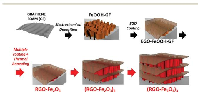
Fig. 1 Schematic illustration of the preparation process for multilayer RGO-Fe<sub>2</sub>O<sub>3</sub> graphitic foam architectures.
