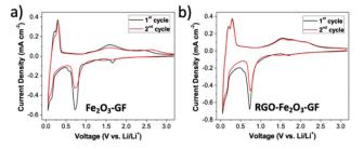
Fig. 6 Cyclic voltammetry curves of (a) Fe<sub>2</sub>O<sub>3</sub>-GF composites and (b) RGO-Fe<sub>2</sub>O<sub>3</sub>-GF composites for the 1<sup>st</sup> and 2<sup>nd</sup> cycles at a scan rate of
