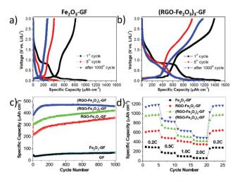
Fig. 7 Charge-discharge profiles of (a) Fe<sub>2</sub>O<sub>3</sub>-GF and (b) (RGO-Fe<sub>2</sub>O<sub>3</sub>)<sub>3</sub>-GF electrodes at 0.2 C. (c) Cycling performance of different electrodes at a charge rate of 2 C. (d) Discharge rate capability of the different electrodes at different discharge rates, after 1000 cycles at 2 C
