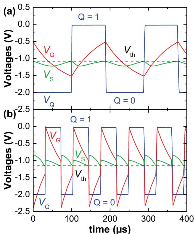
Fig. 2 The measured waveforms in the oscillators in air ambient for  $V_{SS} = -2$  V,  $R_S = 1.26$  k $\Omega$ , and  $C = 1$  nF. (a) The waveforms in the parabolic oscillator with  $R = 85$  k $\Omega$  resulting in the oscillation frequency  $f_{osc} = 5.3$  kHz and duty cycle  $D = 46\%$ . (b) The waveforms in the bow tie oscillator with  $R = 57$  k $\Omega$ ,  $f_{osc} = 13.8$  kHz, and  $D = 55\%$ .
