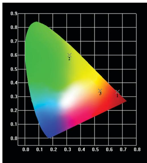
**Fig. 10** 1931 CIE chromaticity diagram of  $(\text{Sm}_{0.5}\text{Gd}_{0.5})_2(\text{BDC})_3(\text{H}_2\text{O})_4$  (3),  $(\text{Eu}_{0.5}\text{Gd}_{0.5})_2(\text{BDC})_3(\text{H}_2\text{O})_4$  (1) and  $(\text{Tb}_{0.5}\text{Gd}_{0.5})_2(\text{BDC})_3(\text{H}_2\text{O})_4$  (2).
