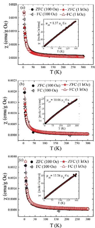
Fig. 12 Temperature dependent dc magnetic susceptibility plots for as-synthesized  $(\text{Ln}_{0.5}\text{Gd}_{0.5})\text{-BDC}$  MOFs. The data shown were collected in the zero-field cooled (ZFC) and field cooled (FC) condition on heating under the applied magnetic field of 100 Oe and 1 kOe for Ln = (a) Sm, (b) Eu and (c) Tb respectively. The insets show the inverse susceptibility plots (black symbols) and the Curie–Weiss fits (red).
