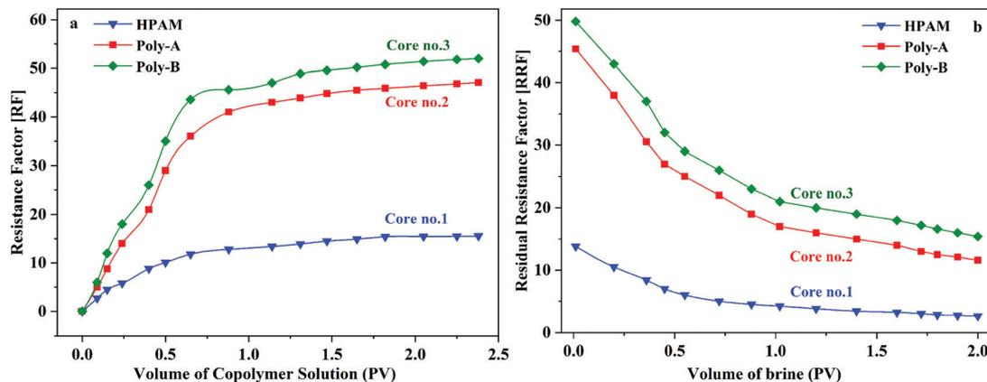
Fig. 10 Flow behavior of copolymer solutions in porous media (copolymer concentration, 2000 mg L<sup>-1</sup>; 70 °C).
