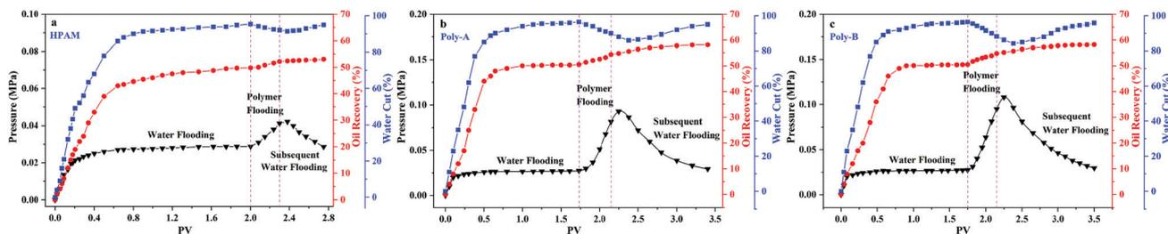
Fig. 11 Core flooding experiments of polymer flooding (copolymer concentration, 2000 mg L<sup>-1</sup>; 70 °C).
