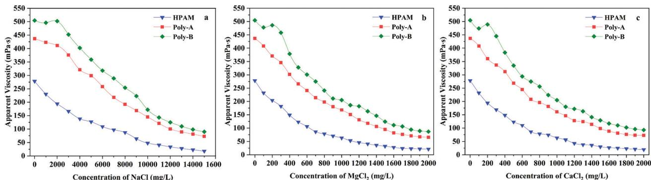
Fig. 8 Salt resistance of copolymers for Na<sup>+</sup>, Mg<sup>2+</sup> and Ca<sup>2+</sup>.
