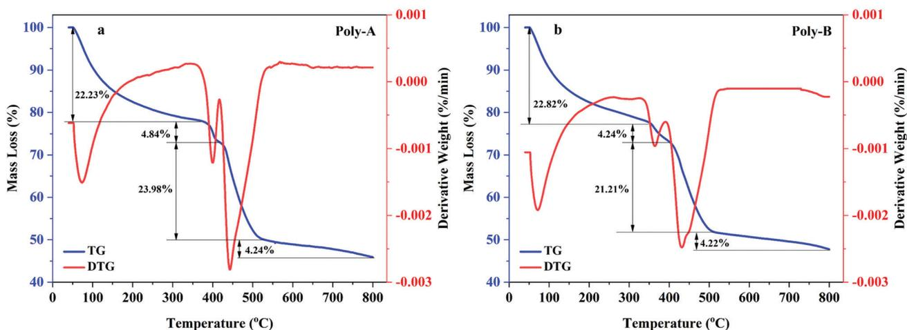
Fig. 4 TG-DTG curves: (a) Poly-A, (b) Poly-B.
