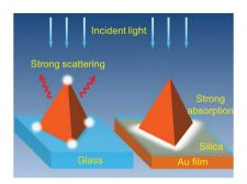
Converting plasmonic light scattering to confined light absorption and creating plexcitons by coupling a gold nano-pyramid array onto a silica-gold film
