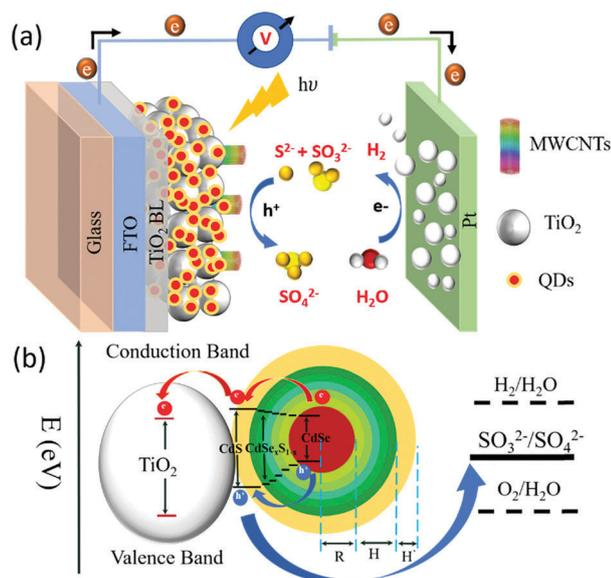
**Fig. 1** Schematic illustration of the: (a) PEC device working principle for  $\text{H}_2$  generation; (b) band structure of the graded alloyed core/shell QDs ( $R$  = radius of CdSe core;  $H$  = thickness of the graded alloyed interfacial layers;  $H'$  = thickness of the outer CdS layer) sensitized  $\text{TiO}_2$ -MWCNT hybrid film applied as the working electrode. The arrows show the electron and hole transfer process.
