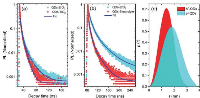
Fig. 4 Comparison of the transient PL curves of heterostructured QDs: (a) deposited onto a ZrO<sub>2</sub> and TiO<sub>2</sub> mesoporous film; (b) deposited onto a ZrO<sub>2</sub> mesoporous film and QDs with electrolyte. The excitation wavelength is  $\lambda_{\text{ex}} = 444$  nm. (c) Comparison of the spatial probability distribution value  $\rho(r)$  of the electron and hole as a function of QD radius  $r$  (nm) ( $H = 2.15$  nm, red for hole and cyan for an electron).
