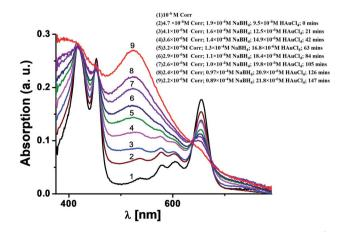
Fig. 2 Time evolution UV-vis spectra of a mixture of 1 ( $\sim$ 10 $^{-6}$ M), NaBH<sub>4</sub> ( $\sim 10^{-4}$ M), and HAuCl<sub>4</sub> ( $\sim 10^{-5}$  M) in DMF.
