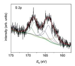
Fig. 8 S 2p spectrum of 1-Au NPs on a Si substrate. Measured data are in black, the fit for bound thiol is in orange, the fit for free thiol is in blue, the fit for oxidized thiol is in dark green, the background is in green and the sum is in red.
