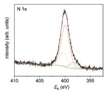
Fig. 7 N 1s XP spectrum of 1-Au NPs on a Si substrate. Measured data are in black, fitted components are in orange, the background is in green and the sum is in red.
