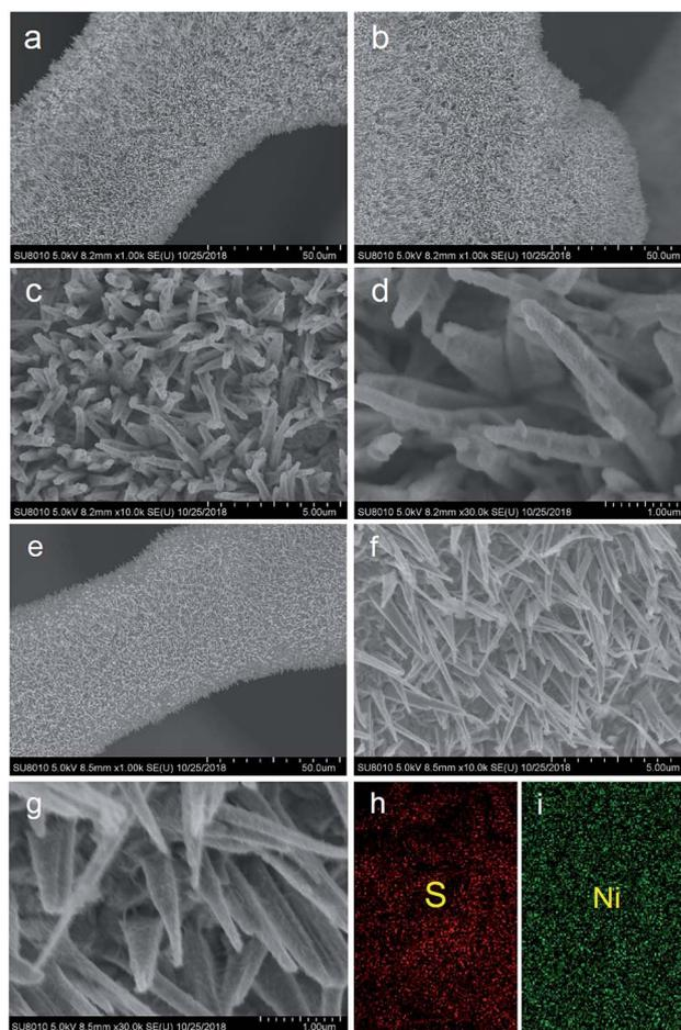
Fig. 2 SEM and EDS images of the Ni<sub>3</sub>S<sub>2</sub> nanorods on Ni foam with different magnifications, (a) and (b) ×1k; (c) ×10k; (d) ×30k; (e) and (f) ×1k; (g) ×10k; (h) EDS image of the S element; (i) EDS image of the Ni element. (a)–(d) images obtained for S-120-16; (e)–(i) images obtained for S-120-18.
