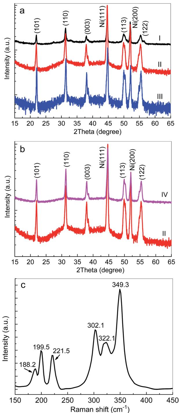
Fig. 1 (a and b) XRD patterns of Ni<sub>3</sub>S<sub>2</sub> nanorods fabricated on Ni foam substrates: (I) 100 °C, 16 h; (II) 120 °C, 16 h; (III) 140 °C, 16 h; (IV) 120 °C, 18 h. (c) The typical Raman spectrum of the Ni<sub>3</sub>S<sub>2</sub> nanorods on Ni foam (S-120-16).
