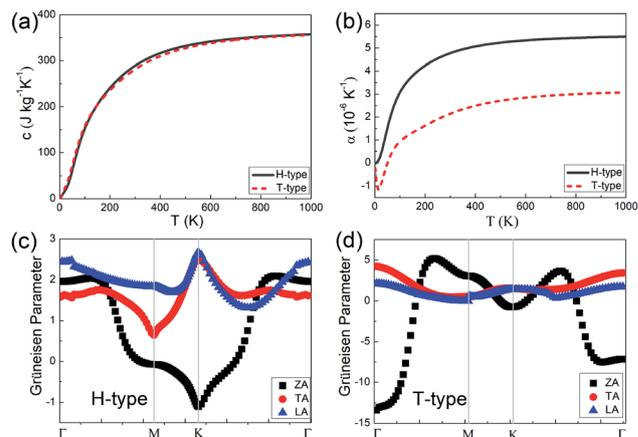
Fig. 4 (a) The specific heats with increasing temperature. (b) The thermal expansion coefficients (TECs) with increasing temperature for both the H- and T-type  $\text{Mo}_2\text{B}$ . (c) and (d) Grüneisen parameters (GPs) in the Brillouin zones (BZs) of the H- and T-type  $\text{Mo}_2\text{B}$ , respectively.
