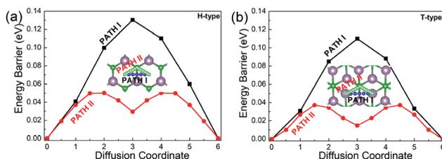
Fig. 5 Diffusion barrier profiles for Li on (a) the H-type  $\text{Mo}_2\text{B}$  and (b) the T-type  $\text{Mo}_2\text{B}$ . The insets show the two migration pathways with low energy barriers on each configuration.
