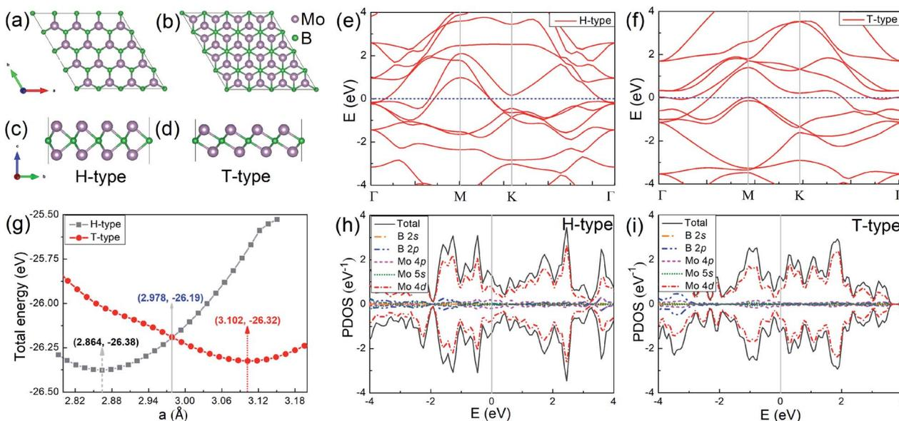
**Fig. 1** (a) and (b) Top-views of the H- and T-type Mo<sub>2</sub>B, respectively; (c) and (d) corresponding side-views for the configurations displayed above. (e) and (f) Electronic energy bands, respectively for the H- and T-type Mo<sub>2</sub>B. (g) Relationships between the total energy and the lattice parameter in the basal plane, for both the H- and T-type structures. (h) and (i) Projected density of states (PDOS), respectively for the H- and T-type Mo<sub>2</sub>B.
