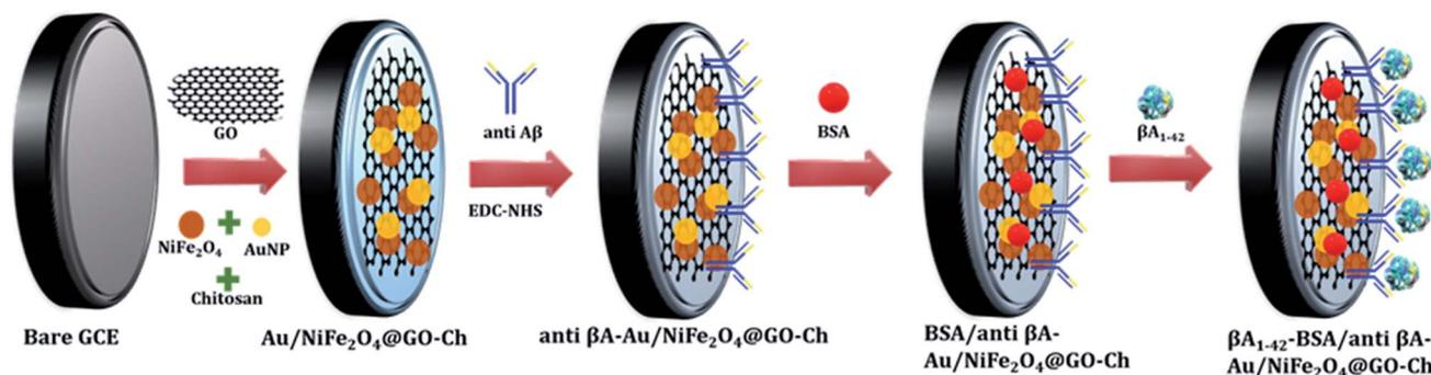
Scheme 1 Schematic representation of fabrication of the immunosensor.
