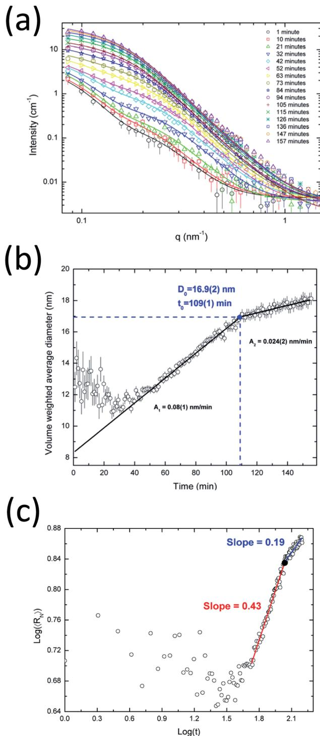
Fig. 5 *In situ* investigations of the synthesis of alloyed silver-gold nanoparticles. (a) Recorded experimental *in situ* SAXS data. The experimental data points (symbols) and theoretical curves (lines) of a few frames are shown for clarity. (b) Evolution of the volume weighted average diameter. (c) log-log plot of the number weighted average radius of the silver-gold nanoalloys as a function of time.
