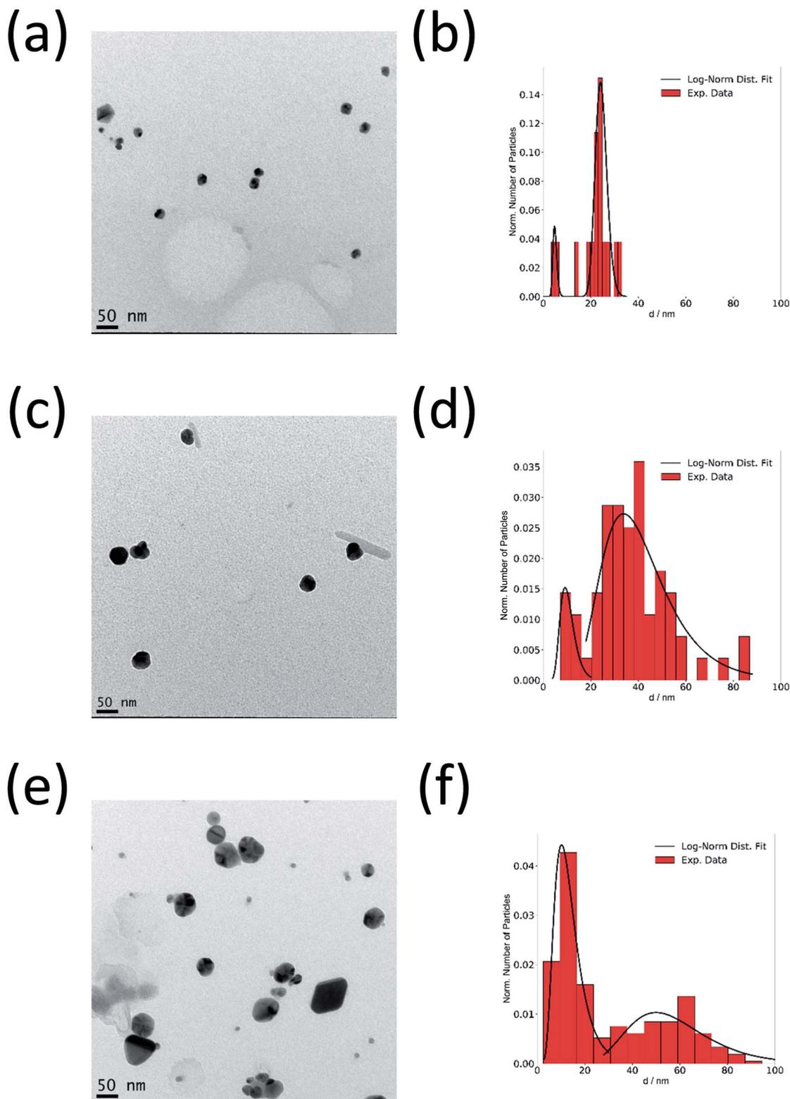
Fig. 3 *Ex situ* TEM investigation of the synthesis of silver nanoparticles at 90 °C. TEM micrographs and particle size distribution of silver nanoparticles obtained after 24 min (a and b), 36 min (c and d) and 72 min (e and f) reaction time.
