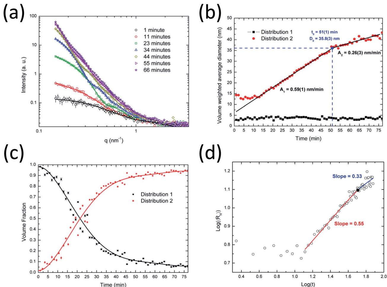
Fig. 2 SAXS results for Ag nanoparticle synthesis. (a) Experimental *in situ* SAXS data (symbols) and theoretical curves (lines) recorded during the synthesis of silver nanoparticles at 90 °C, (b) volume weighted average diameter of distributions 1 and 2, (c) temporal evolution of the volume fractions and (d) log–log plot of the number weighted average radius as a function of time.
