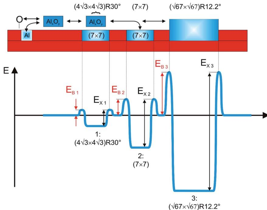
Fig. 8 Qualitative potential diagram of the formation energies per oxygen atom and the related barriers for the formation of the three different surface oxide phases: 1:  $(4\sqrt{3} \times 4\sqrt{3})R30^\circ$  – low temperature double layer oxide, 2:  $(7 \times 7)$  – single layer oxide and 3:  $(\sqrt{67} \times \sqrt{67})R12.2^\circ$  – high temperature double layer oxide.
