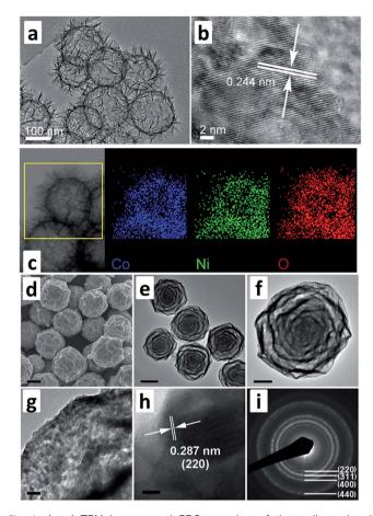
Fig. 1 (a–c) TEM images and EDS mapping of three dimensional  $NiCo_2O_4$  nanospheres, (d–i) SEM and TEM images of seven-layered Ni-Co oxide spheres derived from MOF (modified from ref. 32 and 33, copyright permission from Elsevier and Wiley-VCH, respectively).
