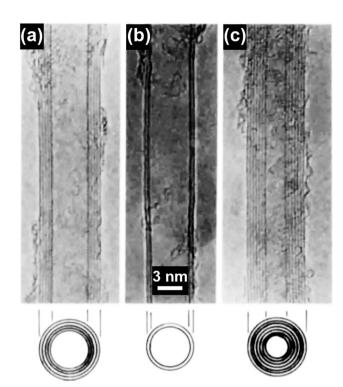
Fig. 1 TEM images of (a) a five-wall CNT, diameter 6.7 nm, (b) a twowall CNT, diameter 5.5 nm, and (c) a seven-wall CNT, diameter 6.5 nm synthesized by arc-discharge. Reproduced from ref. 1, with permission from Nature Publishing Group, 1991.
