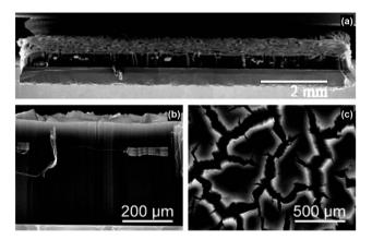
Fig. 8 FE-SEM images of a 420  $\mu$ m thick SWNT film on a 1  $\times$  1 cm silicon wafer substrate prepared by microwave radiation: (a) the overview, (b) cross-sectional view and (c) top view. Reproduced from ref. 59, with permission from Wiley, 2005.
