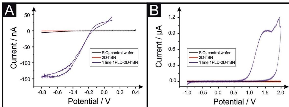
Fig. 1 Cyclic voltammetry for 1 mM RuHex/0.1 M KCl (A) and 1 mM Fe<sup>2+/3+</sup>/0.2 M HClO<sub>4</sub> (B) using a PLD-SiO<sub>2</sub> wafer as first/control (black line), a 2D-hBN electrode (red line) and a PLD-2D-hBN electrode with 1 defective line (blue line) as working electrodes respectively. Scan rate: 50 mV s<sup>-1</sup>; vs. Ag/AgCl. Note that the introduction of a PLD gives rise to an electrochemically useful signature.
