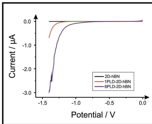
Fig. 5 Linear sweep voltammetry of 2D-hBN, 1PLD-2D-hBN and 6PLD-2D-hBN respectively with  $0.5$  M  $\text{H}_2\text{SO}_4$ , depicting the scanning stability experiments towards the HER; showing an increase in the current when more PLD are created (due to an increase in edge plane-sites/defects) when compared to the bare 2D-hBN electrode (scan rate:  $5$   $\text{mV s}^{-1}$ ; vs. Ag/AgCl).
