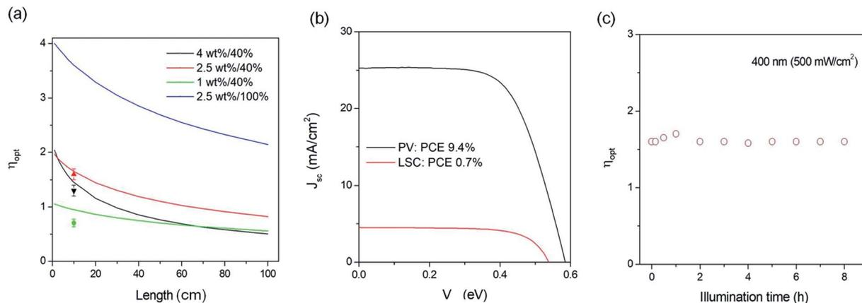
Fig. 5 (a) The calculated and measured external optical efficiency of LSCs based on C-QDs with a QY of 40% and different C-QD concentrations, and a QY of 100% with a concentration of  $3C_0$ . (b)  $J$ - $V$  response of silicon PVs attached on the edge of the LSC under natural sunlight ( $62 \text{ mW cm}^{-2}$ ). (c) The external optical efficiency of LSCs with a C-QD concentration of 2.5 wt% was measured using a power meter upon 400 nm illumination ( $500 \text{ mW cm}^{-2}$ ).
