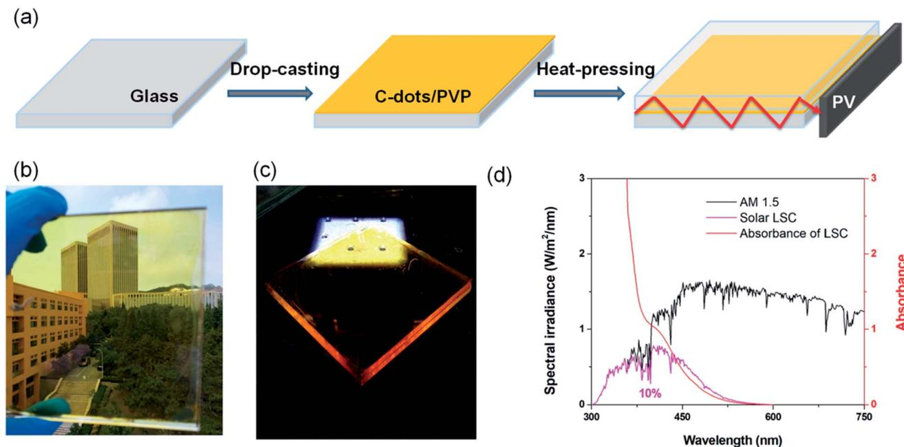
Fig. 3 (a) Scheme of the preparation process for laminated LSCs based on C-QDs. Photographs of the LSC under ambient (b) and one sun ( $100 \text{ mW cm}^{-2}$ ) illumination (c). LSC dimensions,  $10 \times 10 \times 0.9 \text{ cm}^3$ . (d) Absorption and calculated solar absorption of the LSC and solar spectrum (AM 1.5G). The concentration of the C-QDs in PVP was calculated to be 2.5 wt% in PVP based on the data obtained by thermal gravimetric analysis (TGA).
