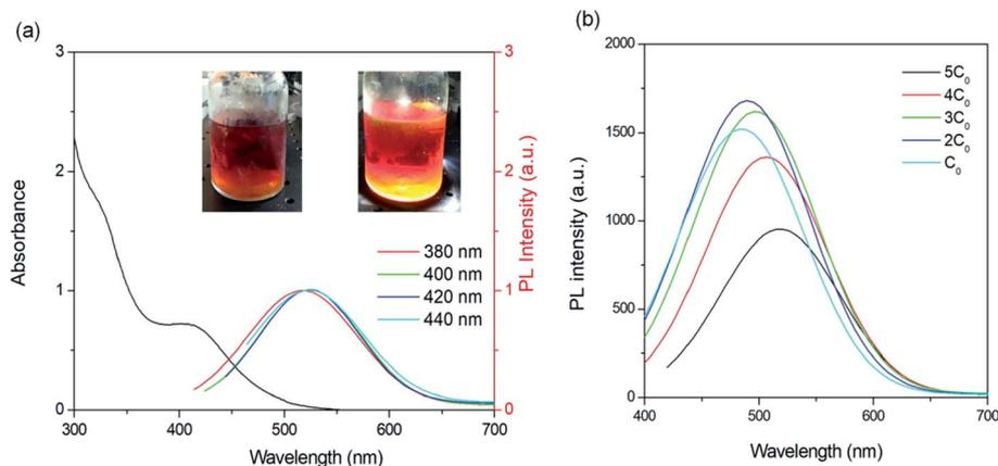
Fig. 2 Absorption and PL spectra of C-QDs dispersed in methanol solution. (b) PL spectra of C-QDs dispersed in methanol solution with different concentrations of C-QDs.  $C_0$  is  $1 \text{ mg mL}^{-1}$ . The excitation wavelength is  $\lambda_{\text{ex}} = 380\text{--}440 \text{ nm}$  for (a) and  $380 \text{ nm}$  for (b). The insets of (a) are the photographs of C-QDs dispersed in methanol under normal conditions (left) and upon simulated sunlight irradiation ( $100 \text{ mW cm}^{-2}$ ).
