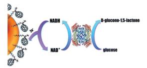
Fig. 7 Working principle of the glucose biosensor based on glucose dehydrogenase, fullerene  $C_{70}$ , and AuNPs. Electrons from glucose are transferred to NAD<sup>+</sup>, fullerene, AuNPs, and finally to the working electrode. Reproduced from ref. 154 – published by The Royal Society of Chemistry.
