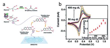
Fig. 6 (a) Chemical reactions that are the basis for the glycerol biosensor operation. Glycerol dehydrogenase (GDH), toluidine blue and electrochemically reduced graphene oxide (ERGO) are deposited on indium-tin oxide (ITO) electrode. Second enzyme (lipase) is not shown. (b) Response studies of the biosensor to varying concentrations of triglyceride (tributyrin). Inset: corresponding calibration curve. Reproduced from ref. 147 with permission from The Royal Society of Chemistry.
