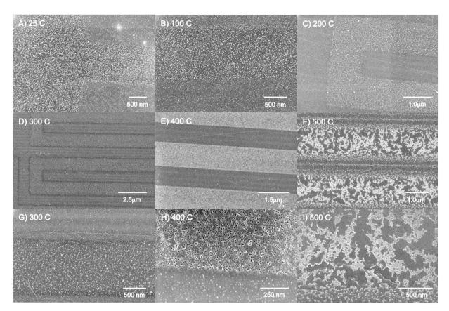
Fig. 2 FESEM images of iron oxide nanoparticles deposited on HOPG at (A) 25 °C and annealed in air, sequentially at (B) 100 °C, (C) 200 °C, (D) 300 °C, (E) 400 °C and (F) 500 °C. Images (G), (H) and (I) are higher magnification images in regions of Figures (D), (E), and (F), respectively.
