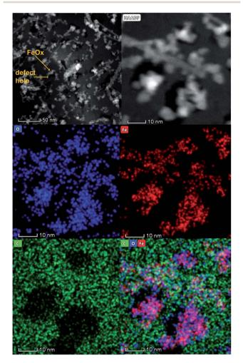
Fig. 7 STEM HAADF images and EDS mapping images of iron oxide particles grown on defects and annealed at 400 °C on a graphene coated TEM grid.
