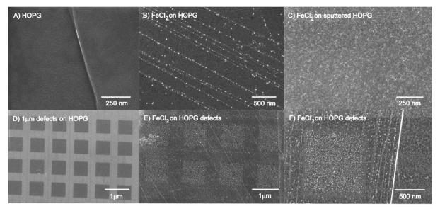
Fig. 1 FESEM images comparing both cleaved HOPG and FIB HOPG defect areas before and after exposure to FeCl<sub>2</sub>(aq): (A) HOPG, (B) iron oxide nanoparticles grown on HOPG, (C) iron oxide nanoparticles grown on Ar<sup>+</sup> sputtered HOPG, (D) FIB HOPG, (E) iron oxide nanoparticles grown on FIB defects on HOPG, and (F) higher magnification image of (E) - note: the white line is iron oxide nanoparticles grown on a step edge across the image
