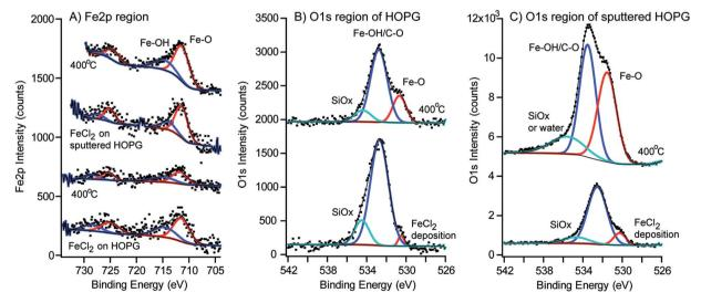
Fig. 6 Fe2p and O1s XPS regions of iron oxide nanoparticles (before and after annealing) on HOPG and Ar<sup>+</sup> sputtered HOPG. (A) Fe2p region of iron oxide nanoparticles on HOPG and  $Ar^+$  sputtered HOPG before and after annealing at 400 °C. The O1s region is shown to compare (B) iron oxide nanoparticles on HOPG after deposition and after annealing at 400 °C with (C) iron oxide nanoparticles on Ar<sup>+</sup> sputtered HOPG after deposition and after annealing at 400 °C.
