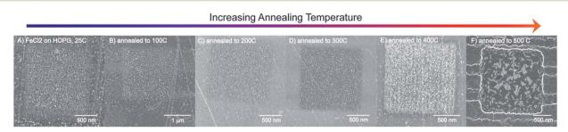
Fig. 3 FESEM images of the annealing profile of iron oxide nanoparticles on HOPG annealed to (A) 25 °C, (B) 100 °C, (C) 200 °C, (D) 300 °C, (E) 400 °C and (F) 500 °C. Iron oxide nanoparticles are shown to coalesce in defect sites of an FIB sputtered HOPG sample by 400 °C. After annealing to 500 °C, the HOPG surface begins to oxidize forming large channels, beginning at the defect (sp<sup>3</sup>) sites.
