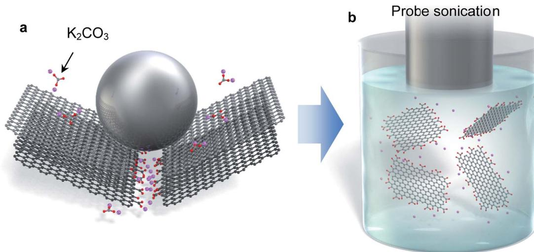
**Fig. 1** Schematic diagram of the mechanochemical reaction and exfoliation of anionic graphene. (a) Carbon radicals are generated by fragmentation of graphite by ball milling. Some salts react with the carbon radicals, forming a functionalized edge. (b) Alkali metals at the edge dissociate in a polar solvent, leading to negative charge. The enhanced electrical repulsion enables exfoliation of graphite in incompatible solvents such as water and alcohol.
