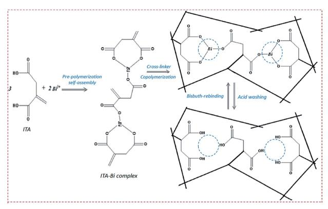
Fig. 21 Schematic representation of Bi<sup>3+</sup>-imprinted polymer synthesis including Bi<sup>3+</sup> interaction with itaconic acid (ITA) molecules (prepolymerization reaction) and copolymerization reaction. Reproduced with permission from ref. 76. Copyright 2017, Elsevier.
