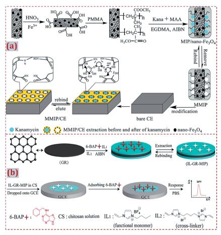
Fig. 8 (a) Schematic of the preparation process of magnetism imprinted electrochemical sensor based on MWCNTs decorated on Fe $_3O_4$  NPs. Reproduced with permission from ref. 103. Copyright 2015, Elsevier. (b) Schematic illustration for the synthesis of IL-GR-MIP composite dropped on GCE and the detection process for the electrochemical sensor. Reproduced with permission from ref. 131. Copyright 2018, Elsevier.
