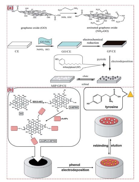
Fig. 6 (a) Detailed procedure diagrams for the fabrication of MIP/GP/CE sensor for 4-nonylphenol. Reproduced with permission from ref. 83. Copyright 2013, Elsevier. (b) Procedures for fabrication of MIP/cAuNPs/2-AETGO/GC sensor for tyrosine detection. Reproduced with permission from ref. 148. Copyright 2015, Elsevier.
