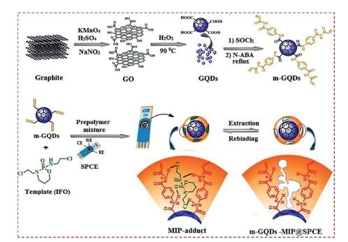
Fig. 7 (a) Schematic illustration for the preparation of monomeric graphene quantum dots (m-GQDs) and fabrication of screen-printed carbon electrode (SPCE) modified with m-GQD-MIP. Reproduced with permission from ref. 88. Copyright 2017, Elsevier.
