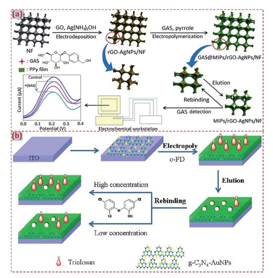
Fig. 3 (a) Schematic illustration of the preparation and application of MIP/rGO-AqNPs/NF sensing system. The control is MIP/rGO-AqNPs/NF without the addition of GAS. Reproduced with permission from ref. 160. Copyright 2018, Elsevier. (b) Schematic of the fabrication of a MIP photoelectrochemical sensor based on g-C<sub>3</sub>N<sub>4</sub>-AuNP-modified ITO electrode. Reproduced with permission from ref. 176. Copyright 2018, Wiley.
