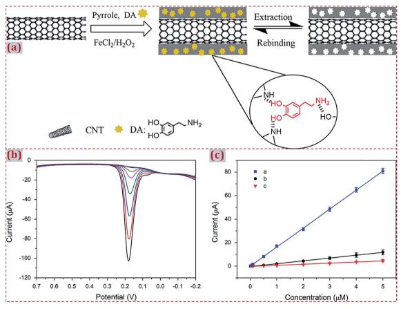
Fig. 17 (a) Chemical routes for the preparation of polypyrrole/CNT-MIP. (b) DPV curves with an increase in DA concentrations in 0.1 M PBS (pH 6.5). DA concentration was 0.05-50 nM and 0.1-5  $\mu$ M (from top to bottom), respectively. (c) Calibration curves of DA obtained with (blue) polypyrrole/CNT-MIP, (black) polypyrrole/CNT-NIP and (red) CNT-modified GCE. Reproduced with permission from ref. 43. Copyright 2014, Elsevier.
