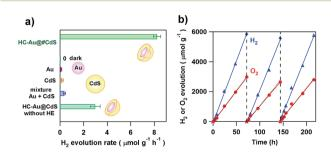
Fig. 5 (a) The comparison of the  $H_2$  evolution rate for HC-Au( $d_{Au}=5.5\,$  nm)@#CdS(lCdS = 1.9 nm), Au colloid, CdS, and a mixture of Au and CdS under red-light illumination ( $\lambda_{ex}=640\,$  nm) or dark conditions. (b) Repeated water splitting by HC-Au( $d_{Au}=12.1\,$  nm) @#CdS(lCdS = 2.1 nm) under red-light illumination. Figures are taken from ref. 59.
