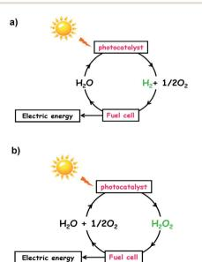
Scheme 1 (a) Solar hydrogen cycle and (b) solar oxygen cycle.
