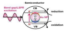
Fig. 2 Local electromagnetic field-enhanced mechanism.
