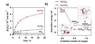
Fig. 4 Time courses for the M(Au and Pt)/TiO<sub>2</sub>-photocatalyzed ORR to  $H_2O_2$  under UV-light irradiation ( $\lambda > 300$  nm, light intensity  $I_{290-390~\rm nm} = 3$  mW cm<sup>-2</sup>) and unmodified TiO<sub>2</sub> system for comparison. (b) Adsorption energy change with the  $M_{28}/{\rm TiO_2}$ -photocatalyzed two-electron ORR (M = Au and Pt. Figure (b) is taken from ref. 54.
