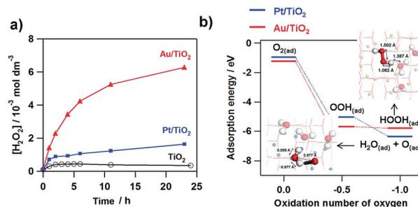
Fig. 4 Time courses for the M(Au and Pt)/TiO<sub>2</sub>-photocatalyzed ORR to H<sub>2</sub>O<sub>2</sub> under UV-light irradiation ( $\lambda > 300 \text{ nm}$ , light intensity  $I_{290-390 \text{ nm}} = 3 \text{ mW cm}^{-2}$ ) and unmodified TiO<sub>2</sub> system for comparison. (b) Adsorption energy change with the M<sub>28</sub>/TiO<sub>2</sub>-photocatalyzed two-electron ORR (M = Au and Pt. Figure (b) is taken from ref. 54.
