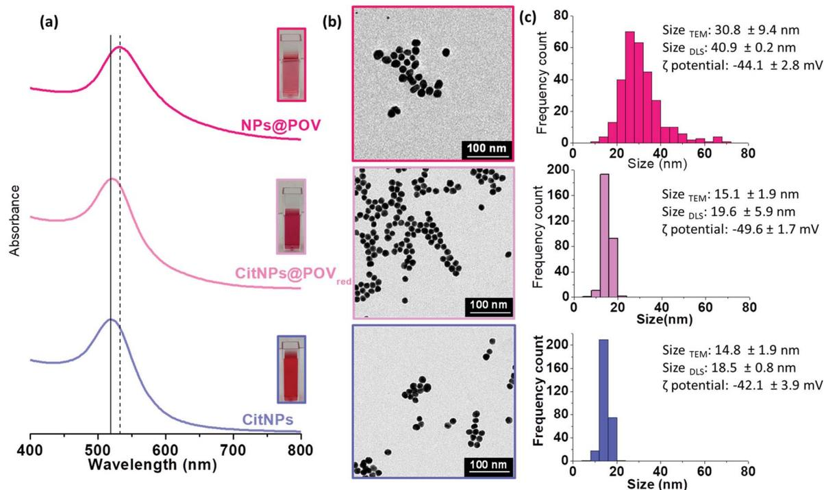
Fig. 2 Characterization of CitNPs, CitNPs@ $\text{POV}_{\text{red}}$  and NPs@POV. UV-vis spectra and colloidal suspension pictures (inset) (a), TEM images (b) and particle size distribution histograms and dynamic light scattering size and zeta potential values (c).
