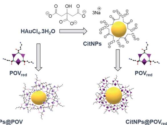
Scheme 1 Schematic representation of CitNPs, CitNPs@POV<sub>red</sub> and NPs@POV synthesis.
