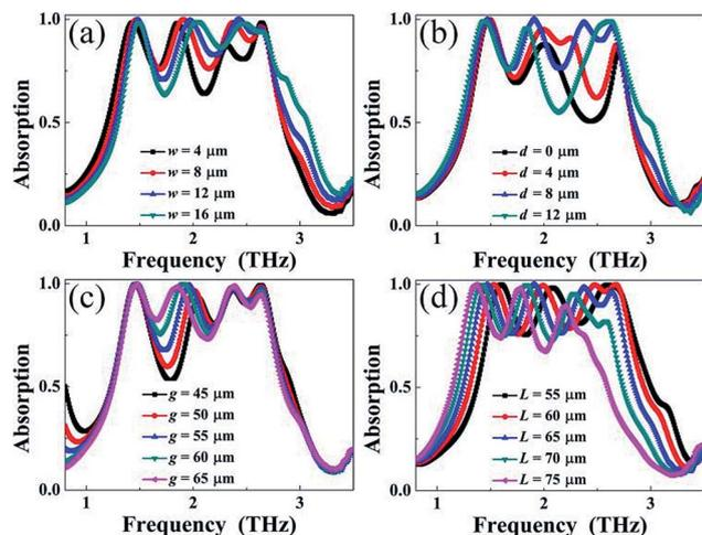
Fig. 5 Resonance absorption spectra of the suggested broadband PMA as a function of frequency with changes in different parameters such as the (a) slot length  $w$ , (b) slot deviation value  $d$ , (c) slot width  $g$ , and (d) entire resonator length  $L$ .
