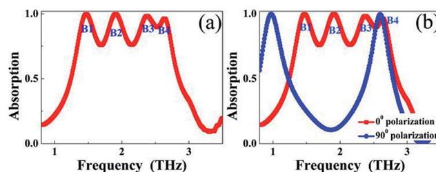
Fig. 2 (a) Resonance absorption spectra of the broadband PMA as a function of frequency; (b) resonance absorption spectra of the broadband PMA as a function of frequency at two different polarization angles.
