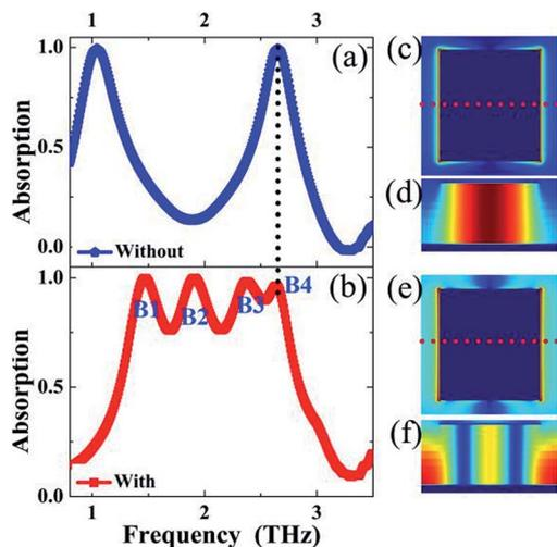
Fig. 3 Resonance absorption response of the Au resonator without (a) or with (b) the elongated slot; the electric ( $|E|$ , in the resonator central plane) fields of the first (c) and second (e) frequency points of Fig. 3(a); the magnetic ( $|H_y|$ , perpendicular to the resonator along the red dotted line) fields of the first (d) and second (f) frequency points of Fig. 3(a).
