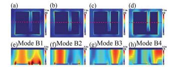
Fig. 4 The electric (|E|, in the resonator central plane) fields of the frequency points B1 (a), B2 (b), B3 (c), and B4 (d); the magnetic ( $|H_y|$ , perpendicular to the resonator along the red dotted line) fields of the frequency points B1 (e), B2 (f), B3 (g), and B4 (h).
