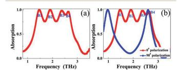
Fig. 2 (a) Resonance absorption spectra of the broadband PMA as a function of frequency; (b) resonance absorption spectra of the broadband PMA as a function of frequency at two different polarization angles
