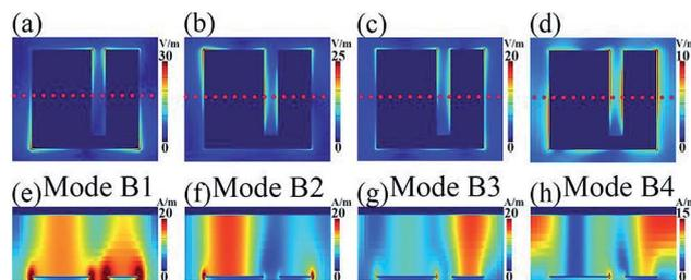
Fig. 4 The electric ( $|E|$ , in the resonator central plane) fields of the frequency points B1 (a), B2 (b), B3 (c), and B4 (d); the magnetic ( $|H_y|$ , perpendicular to the resonator along the red dotted line) fields of the frequency points B1 (e), B2 (f), B3 (g), and B4 (h).
