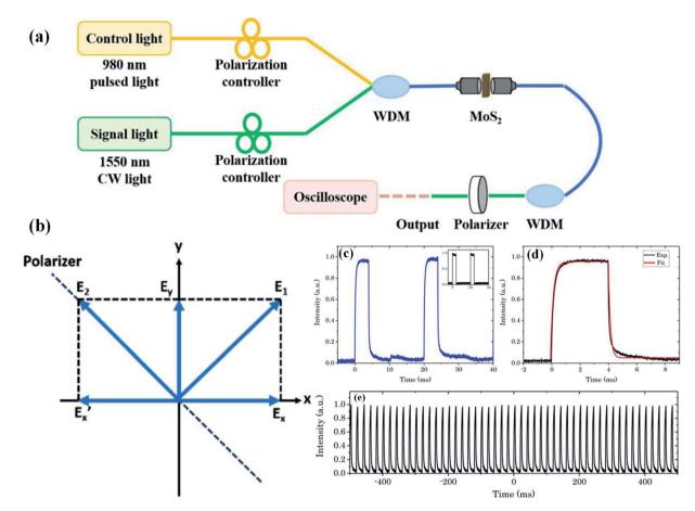
Fig. 7 (a) A PI fiber all-optical modulator based MoS<sub>2</sub>-PVA thin films. (b) Device principle. (c) Waveform of signal light, inset: waveform of control light (pump). (d) A zoomed view of a single off-on-off transition of the signal light and the corresponding fitting curve. (e) Output signal light in a long-time region. This figure has been adapted from ref. 13 and 96 with permission from Chinese Optics Letters, Photonics Research.
