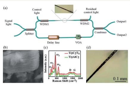
Fig. 2 (a) Experimental setup of an MZI all-optical modulator based on MXene materials. (b) High-resolution electron microscopy image of MXene nanosheets. (c) Raman spectrum of  $Ti_3AlC_2$  and  $Ti_3C_2T_x$ . (d) Optical microscopy image of microfibers deposited with MXenes. This figure has been adapted from ref. 16 with permission from Advanced Materials
