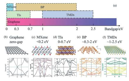
Fig. 1 (a) Distribution diagram of the bandgap of 2D materials. The atomic structures and band structures (monolayer) of graphene, (b) MXene, (c) TIs, (d) BP (e) and TMDs (f). This figure has been adapted from ref. 37, 61, 69 and 76 with permission from Nature Physics, Advanced Materials, Nature Photonics, Journal of the American Chemical Society.
