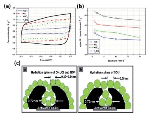
Fig. 8 (a) Cyclic voltammograms of activated CCDC supercapacitors in the aqueous electrolytes 0.5 M K<sub>2</sub>SO<sub>4</sub>, 2 M KCl, 1 M KNO<sub>3</sub> and 6 M KOH  $(20 \text{ mV s}^{-1})$  and (b) the specific capacitance of the supercapacitor at different scan rates. (c) Schematic diagram of the relationship of hydration sphere ions and pores. This figure has been adapted from ref. 115 with permission from Elsevier.
