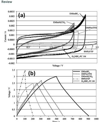
Fig. 18 (a) CV of various electrolytes at  $5 \text{ mV s}^{-1}$  and (b) galvanostatic charge–discharge at  $2 \text{ mA cm}^{-2}$ . This figure has been adapted from ref. 168 with permission from the Royal Society of Chemistry.
