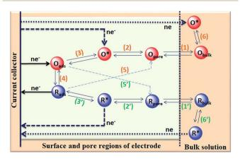
Fig. 23 Illustration of charge storage mechanisms in the porous carbon electrode of a supercapacitor with a redox electrolyte.
