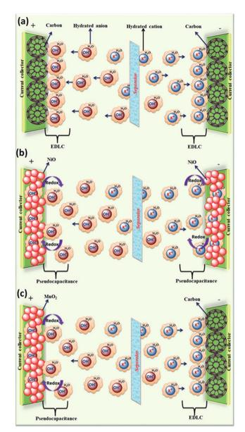
Fig. 6 Graphical representation of reaction mechanism between alkaline electrolyte (KOH) and carbon– $MnO_2$  electrodes for (a) EDLC (b) pseudocapacitor (c) hybrid supercapacitor.
