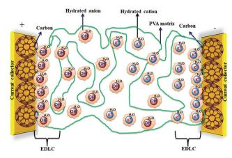
Fig. 19 Graphical representation of a hydrogel polymer electrolyte (PVA/KOH/ $\rm H_2O$ ) and a carbon electrode for EDLCs.
