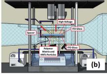
Fig. 1 (a) Real-time solution drying platform which measures changes in out-of-plane and in-plane retardation along with thickness, weight and temperature; (b) modified setup to measure birefringence response on electric field application.
