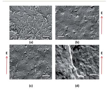
Fig. 10 (a) Morphology of halloysite particles, (b) 2 wt%, (c) 4 wt% and (d) 6 wt% treated HNTs aligned in the matrix under an electric field strength of 700 V mm $^{-1}$  at 100 Hz (scale bar = 2  $\mu$ m).
