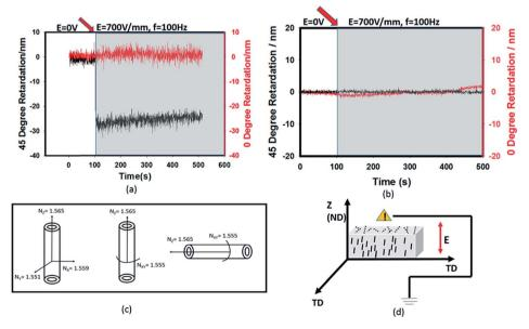
Fig. 2 Response of 0° and 45° retardation on the application of an electric field at 100 seconds on (a) 4 wt% HNT loading system with an applied electric field of 700 V mm $^{-1}$  at 100 Hz; (b) pure photocurable resin; (c) schematic of  $N_{xy}$  and  $N_z$  of HNTs; (d) schematic of the HNTs oriented in polymer films. Double arrow indicates the direction of the electric field.
