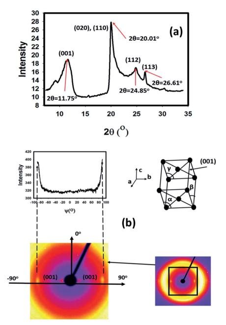
Fig. 7 (a) WAXD spectra for modified HNTs, (b) Azimuthal scan of the WAXS pattern of the 4 wt% HNT nanocomposite and unit cell of the halloysite nanotube crystal and its (001) plane
