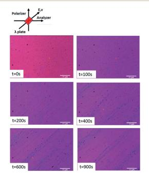
Fig. 6 Time sequence images showing alignment of HNTs in the electric field (700 V mm $^{-1}$ , 100 Hz) with the electric field parallel to the slow axis of the red wave  $\lambda$  plate.
