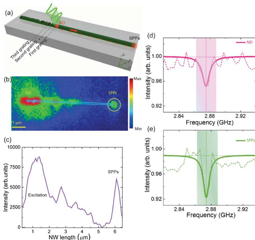
**Fig. 3** (a) Schematic of the NW-OGC system based on a MPTMS adhesion layer coupled to the NV centre in NDs showing a map of the variable displacement of the ND. The corresponding photon emission map and intensity profile are shown in (b) and (c), respectively. Measurement of the NV spin state readout in a ND coupled NW-OGC system showing a reduction in the photoluminescence intensity in ND emission (d) and a reduction in the SPP scattering strength (e).
