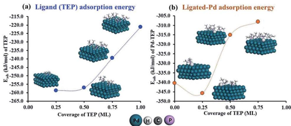
Fig. 7 (a) Adsorption energy ( $E_{\text{ads}}$ ) of triethylphosphine at coverages from 0.25 ML to 1 ML on Pd(111); (b) adsorption energy of Pd–TEP (where a single Pd atom is coordinated with triethylphosphine through a Pd–P bond) vs. TEP coverage on Pd(111). Color code for atoms: Pd–teal, H–white, C–grey, and P–magenta. Adsorbed Pd atoms are shown in light grey.
