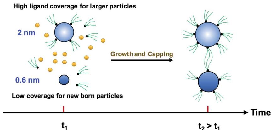
Fig. 4 Schematic diagram for the growth and capping of two different sized populations. The metal precursor and ligands are shared among 0.6 nm (new born nanoparticles) and 2 nm nanoparticles. Additional nucleation events are not shown for clarity; however, continuous nucleation is accounted for in this approach by adding more nuclei (0.6 nm) overtime as described in the text.
