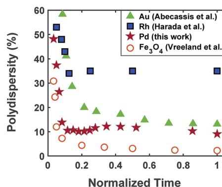
Fig. 3 Polydispersity as a function of normalized reaction time for Au (Abecassis *et al.*<sup>39</sup> (acidic ligand)), Rh (Harada *et al.*<sup>46</sup> (without NaCl)), Pd (our work), and Fe<sub>3</sub>O<sub>4</sub> (Vreeland *et al.*<sup>27</sup>). Normalized time is defined as: time (experimental data collected)/time (end of reaction).
