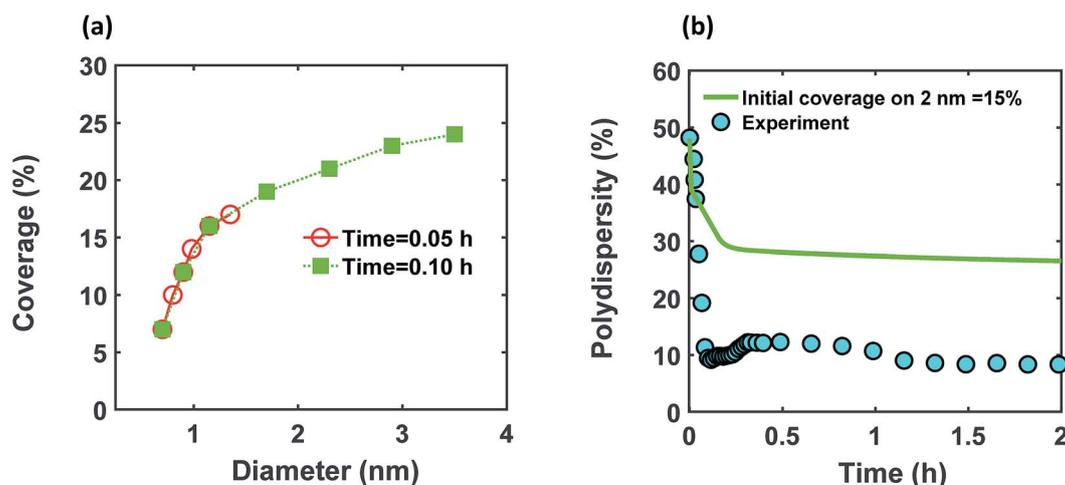
Fig. 5 (a) Model prediction of coverage vs. nanoparticle diameter at time = 0.05 and 0.10 h; a (b) time evolution of polydispersity ( $P(t) = \frac{\sigma(t)}{D_{ave}(t)}$ ). At time zero, the 2 nm nanoparticle population has 15% initial ligand coverage, while the initial coverage of smaller size population; 0.6 nm, is zero. Experimental conditions: 10 mM Pd(OAc)<sub>2</sub> in 1 : 1 pyridine/hexanol, TOP : Pd = 1, and  $T = 100^\circ\text{C}$ .
