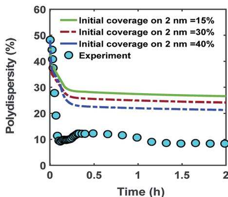
Fig. 6 Effect of initial ligand coverage at time zero (15, 30 and 40%) of the larger size (2 nm) population on the time evolution of polydispersity  $\left(P(t) = \frac{\sigma(t)}{D_{ave}(t)}\right)$  in the case of continuous nucleation. The maximum coverage for the cases with 15%, 30%, and 40% initial ligand coverage on 2 nm nanoparticles is 32%, 45%, and 55%, respectively. Nucleation rate (model = experiment).
