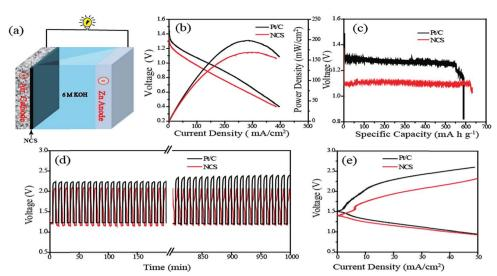
Fig. 6 (a) Schematic structure of the Zn-air battery, (b) I-V polarization curves of the battery by using NCS and Pt/C as the cathode materials, (c) typical discharge curves of the Zn-air battery under continuous discharge until complete consumption of Zn, (d) charge-discharge cycles performed at a current density of 10 mA cm<sup>-2</sup> and (e) charging and discharging polarization (I-V) plots of the rechargeable Zn-air battery.
