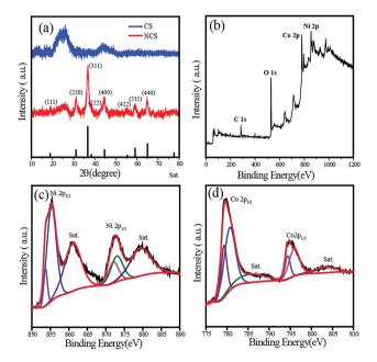
Fig. 3 (a) XRD spectra of NCS and CS; (b) XPS survey spectrum representing the elements in NCS; (c) and (d) deconvoluted Ni2p and Co2p XPS spectra of NCS.
