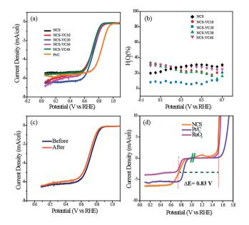
Fig. 5 (a) Linear sweep voltammograms (LSVs) recorded for all the catalysts in 0.1 M KOH at an electrode rotation speed of 1600 rpm, (b) the amount of  $\rm H_2O_2$  calculated as a function of the electrode potential from RRDE, (c) LSVs of NCS recorded before and after ADT and (d) the plot representing the bifunctional catalytic activities of NCS toward the ORR and OER.
