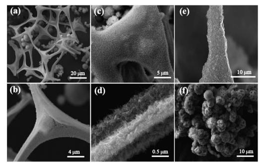
Fig. 1 (a and b) Low magnification FESEM images of NCS showing the interconnected three-dimensional network, (c and d) high magnification FESEM images presenting the nanoarray of NiCo<sub>2</sub>O<sub>4</sub> over the CS surface, (e) FESEM image of the CS surface and (f) FESEM image of the NiCo<sub>2</sub>O<sub>4</sub> flower bundle structure formed in the reaction with CN.
