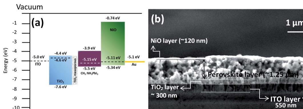
Fig. 6 (a) Energy band alignment of the structure consisting of glass/ITO/TiO<sub>2</sub> compact layer/TiO<sub>2</sub> mesoporous layer/CH<sub>3</sub>NH<sub>3</sub>PbI<sub>3</sub>/NiO NCs layer/Au. (b) Cross sectional image of the device (glass/ITO/TiO<sub>2</sub> compact layer/TiO<sub>2</sub> mesoporous layer/CH<sub>3</sub>NH<sub>3</sub>PbI<sub>3</sub>/NiO) without the metal contact (Au) showing the thicknesses of each layer.
