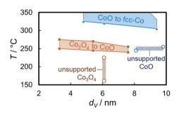
Fig. 10 Temperature ranges for a 1 °C min<sup>-1</sup> ramp rate of the reduction of exfoliated graphite-supported (5 wt% Co) and unsupported Co<sub>3</sub>O<sub>4</sub> crystallites to CoO and the subsequent reduction to metallic Co in hydrogen as observed via in situ X-ray diffraction as a function of the volume-mean crystallite size as obtained from Rietveld refinement.
