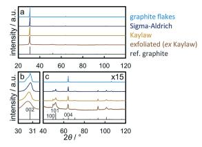
Fig. 2 (a) Normalised X-ray diffraction patterns, (b) enlarged (002) reflections, and (c) the patterns above 40° with 15 times increased intensities of graphitic materials with a reference pattern for graphite.
