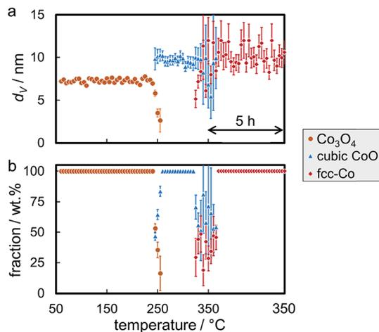
Fig. 7 (a) Volume-mean crystallite sizes and (b) weight fractions with the particular errors of the phases as obtained *via* Rietveld refinement of *in situ* X-ray diffraction patterns during reduction of 5 wt% Co<sub>7.6</sub> on exfoliated graphite in hydrogen at 350 °C for 5 h.
