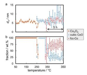
Fig. 8 (a) Volume-mean crystallite sizes and (b) weight fractions with the particular errors of the phases as obtained *via* Rietveld refinement of *in situ* X-ray diffraction patterns during reduction of 5 wt% Co\_4.9 on exfoliated graphite in hydrogen at 350 °C for 5 h.
