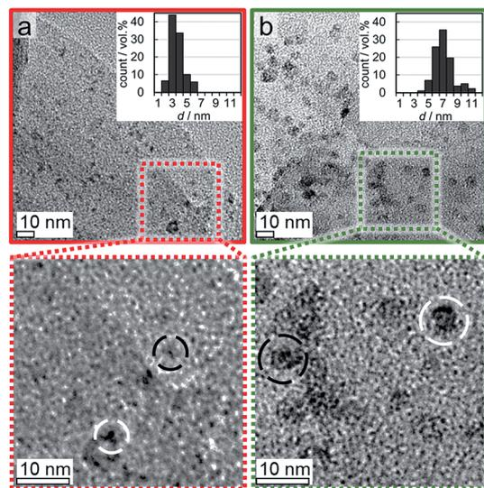
**Fig. 16** Transmission electron micrographs of 1 wt% (a) Co<sub>3.5</sub> and (b) Co<sub>7.6</sub> on exfoliated graphite after reduction in hydrogen at 350 °C and 330 °C, respectively, during *in situ* X-ray diffraction with volume-based size distribution and enlarged areas displaying reduced and passivated crystallites of unchanged sizes (encircled black) and after sintering (encircled white).
