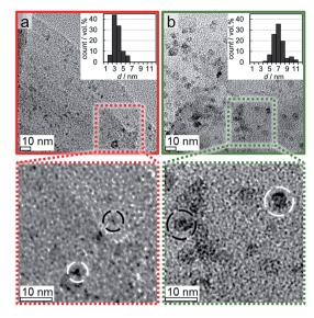
**Fig. 16** Transmission electron micrographs of 1 wt% (a) Co\_3.5 and (b) Co\_7.6 on exfoliated graphite after reduction in hydrogen at 350 °C and 330 °C, respectively, during *in situ* X-ray diffraction with volume-based size distribution and enlarged areas displaying reduced and passivated crystallites of unchanged sizes (encircled black) and after sintering (encircled white).
