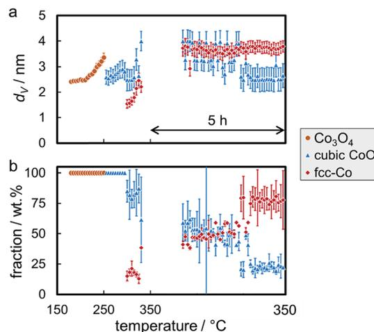
Fig. 15 (a) Volume-mean crystallite sizes and (b) weight fractions with the particular errors of the phases as obtained *via* Rietveld refinement of synchrotron radiation-based *in situ* X-ray diffraction patterns during reduction of 1 wt% Co<sub>3.5</sub> on exfoliated graphite in hydrogen at 350 °C for 5 h.
