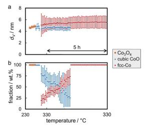
Fig. 14 (a) Volume-mean crystallite sizes and (b) weight fractions with the particular errors of the phases as obtained via Rietveld refinement of synchrotron radiation-based in situ X-ray diffraction patterns during reduction of 1 wt% Co\_7.6 on exfoliated graphite in hydrogen at 330 °C for 5 h.
