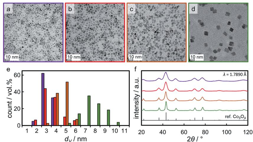
Fig. 4 (a–d) Transmission electron micrographs of the Co<sub>3</sub>O<sub>4</sub> nanoparticles obtained in synthesis Co<sub>2.8</sub>, Co<sub>3.5</sub>, Co<sub>4.9</sub>, and Co<sub>7.6</sub>, respectively, together with (e) the particular volume-based size distributions and (f) X-ray diffractograms with a reference pattern for Co<sub>3</sub>O<sub>4</sub>. In part reproduced from ref. 9 with permission from The Royal Society of Chemistry.
