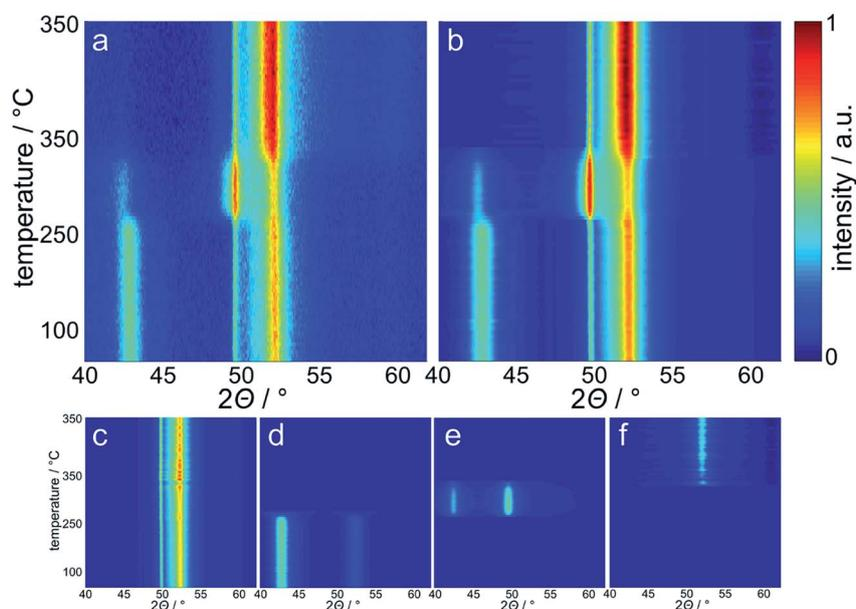
Fig. 6 Top-view of (a) the experimentally obtained *in situ* X-ray diffraction patterns during reduction of 5 wt% Co<sub>7.6</sub> on exfoliated graphite in hydrogen at 350 °C for 5 h, (b) calculated patterns obtained *via* Rietveld refinement with the background being deducted and the corresponding fitted contributions of (c) the summed-up exfoliated graphite phases from PONKCS analysis, (d) Co<sub>3</sub>O<sub>4</sub>, (e) cubic CoO, and (f) fcc-Co.
