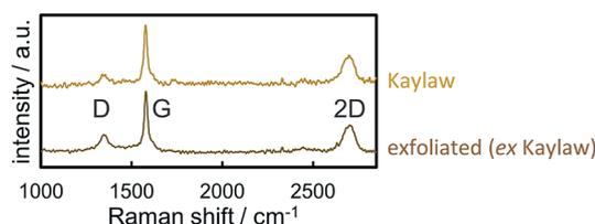
**Fig. 3** Raman spectra of pristine and exfoliated Kaylaw graphite powder displaying carbon characteristic bands.
