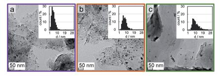
Fig. 11 Transmission electron micrographs and number-based crystallite size distributions of 5 wt% (a) Co\_2.8, (b) Co\_4.9, and (c) Co\_7.6 on exfoliated graphite after reduction in hydrogen at 350 °C during in situ X-ray diffraction.
