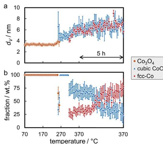
Fig. 9 (a) Volume-mean crystallite sizes and (b) weight fractions with the particular errors of the phases during reduction of 5 wt% Co<sub>2.8</sub> on exfoliated graphite in hydrogen at 370 °C for 5 h, as obtained *via* Rietveld refinement of the *in situ* X-ray diffraction patterns.
