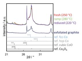
Fig. 13 Synchrotron radiation-based ( $\lambda = 0.9941 \text{ Å}$ ) X-ray diffraction patterns of 1 wt% Co\_7.6 on exfoliated graphite before reduction in hydrogen (fresh), during the initial ramp at 280 °C displaying the maximum concentration of CoO, and after reduction at 330 °C normalised to the (004) reflection of exfoliated graphite (34.2°) with the pattern of exfoliated graphite and reference patterns for fcc-Co, hcp-Co, cubic CoO, and Co<sub>3</sub>O<sub>4</sub>.
