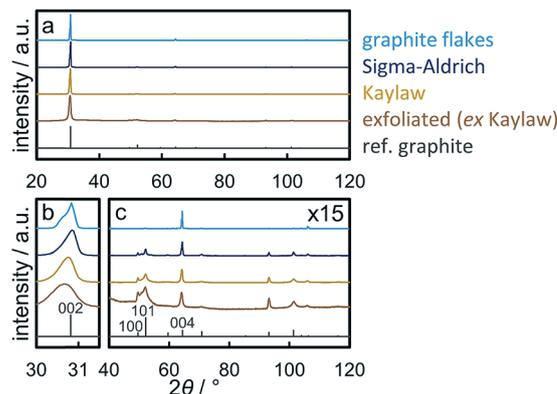
Fig. 2 (a) Normalised X-ray diffraction patterns, (b) enlarged (002) reflections, and (c) the patterns above  $40^\circ$  with 15 times increased intensities of graphitic materials with a reference pattern for graphite.
