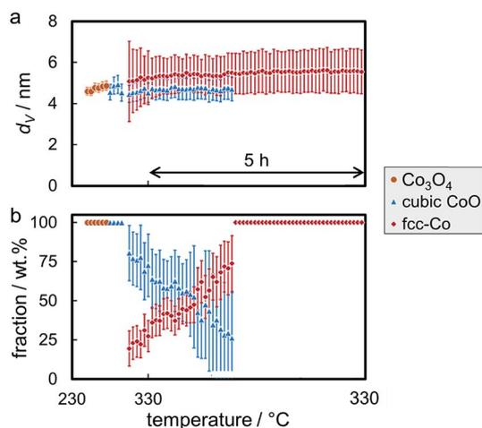
Fig. 14 (a) Volume-mean crystallite sizes and (b) weight fractions with the particular errors of the phases as obtained *via* Rietveld refinement of synchrotron radiation-based *in situ* X-ray diffraction patterns during reduction of 1 wt% Co<sub>7.6</sub> on exfoliated graphite in hydrogen at 330 °C for 5 h.
