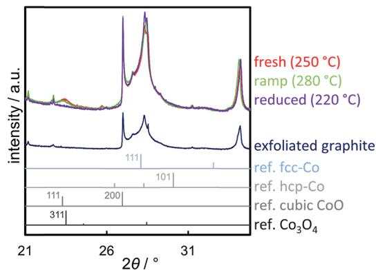
Fig. 13 Synchrotron radiation-based ( $\lambda = 0.9941 \text{ \AA}$ ) X-ray diffraction patterns of 1 wt% Co<sub>7.6</sub> on exfoliated graphite before reduction in hydrogen (fresh), during the initial ramp at 280 °C displaying the maximum concentration of CoO, and after reduction at 330 °C normalised to the (004) reflection of exfoliated graphite (34.2°) with the pattern of exfoliated graphite and reference patterns for fcc-Co, hcp-Co, cubic CoO, and Co<sub>3</sub>O<sub>4</sub>.
