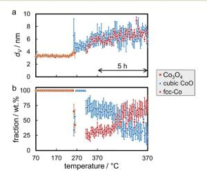
Fig. 9 (a) Volume-mean crystallite sizes and (b) weight fractions with the particular errors of the phases during reduction of 5 wt% Co\_2.8 on exfoliated graphite in hydrogen at 370 °C for 5 h, as obtained *via* Rietveld refinement of the *in situ* X-ray diffraction patterns.
