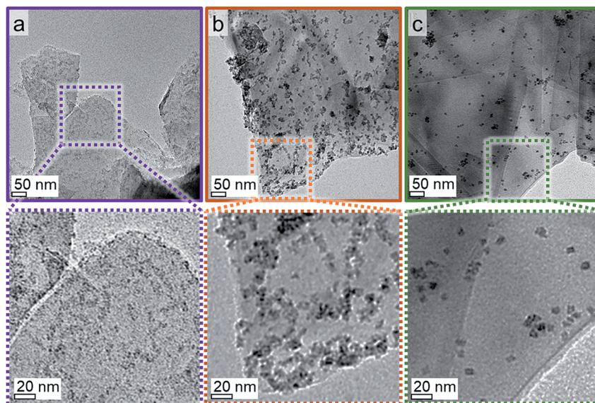
Fig. 5 Transmission electron micrographs of 5 wt% (a) Co<sub>2.8</sub>, (b) Co<sub>4.9</sub>, and (c) Co<sub>7.6</sub> on exfoliated graphite with magnified insets.
