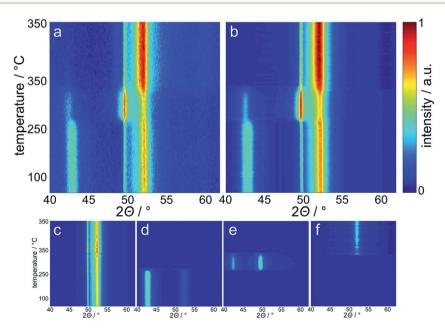
Fig. 6 Top-view of (a) the experimentally obtained in situ X-ray diffraction patterns during reduction of 5 wt% Co\_7.6 on exfoliated graphite in hydrogen at 350 °C for 5 h, (b) calculated patterns obtained via Rietveld refinement with the background being deducted and the corresponding fitted contributions of (c) the summed-up exfoliated graphite phases from PONKCS analysis, (d)  $Co_3O_4$ , (e) cubic CoO, and (f) fcc-Co.
