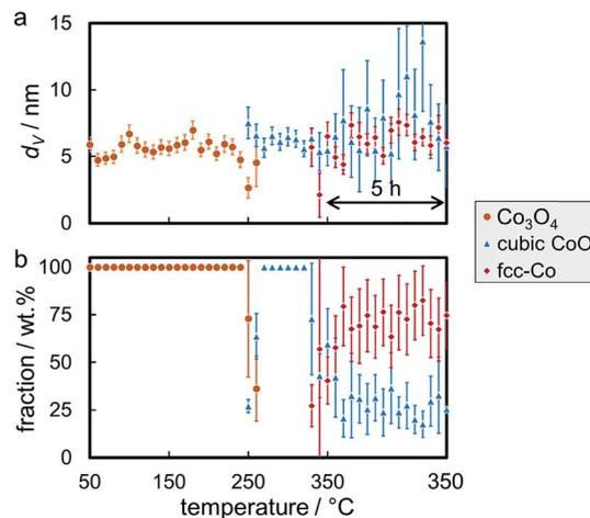
Fig. 8 (a) Volume-mean crystallite sizes and (b) weight fractions with the particular errors of the phases as obtained *via* Rietveld refinement of *in situ* X-ray diffraction patterns during reduction of 5 wt% Co<sub>4.9</sub> on exfoliated graphite in hydrogen at 350 °C for 5 h.
