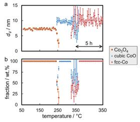
Fig. 7 (a) Volume-mean crystallite sizes and (b) weight fractions with the particular errors of the phases as obtained via Rietveld refinement of  $in\ situ\ X$ -ray diffraction patterns during reduction of 5 wt% Co\_7.6 on exfoliated graphite in hydrogen at 350 °C for 5 h.
