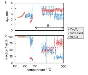
Fig. 15 (a) Volume-mean crystallite sizes and (b) weight fractions with the particular errors of the phases as obtained via Rietveld refinement of synchrotron radiation-based in situ X-ray diffraction patterns during reduction of 1 wt% Co\_3.5 on exfoliated graphite in hydrogen at 350 °C for 5 h.
