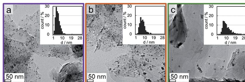
Fig. 11 Transmission electron micrographs and number-based crystallite size distributions of 5 wt% (a)  $\text{Co}_{2.8}$ , (b)  $\text{Co}_{4.9}$ , and (c)  $\text{Co}_{7.6}$  on exfoliated graphite after reduction in hydrogen at 350 °C during *in situ* X-ray diffraction.
