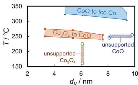
Fig. 10 Temperature ranges for a  $1\text{ °C min}^{-1}$  ramp rate of the reduction of exfoliated graphite-supported (5 wt% Co) and unsupported  $\text{Co}_3\text{O}_4$  crystallites to  $\text{CoO}$  and the subsequent reduction to metallic Co in hydrogen as observed *via in situ* X-ray diffraction as a function of the volume-mean crystallite size as obtained from Rietveld refinement.
