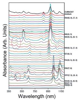
Fig. 9 Absorbance spectra of sequential chromatographically-separated SWCNT populations using a CCC instrument. The emergence and disappearance of absorbance features is due to the differential partitioning of the different SWCNT species along an SDS % gradient starting from a low concentration at the bottom of the figure to high concentration near the top. Reprinted with permission from Zhang et al., Anal. Chem., 2014, 86, 3980–3984. Copyright 2014 American Chemical Society.
