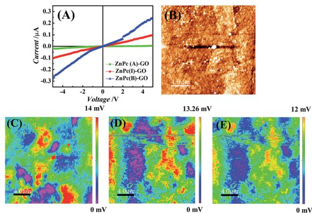
Fig. 6 (A) *I*-*V* curve measurements of the ZnPc(A)-GO, ZnPc(I)-GO and ZnPc(B)-GO samples. (B) AFM topography image of ZnPc-GO over an ITO-coated glass substrate. The KPFM images or surface potential mapping of the (C) ZnPc(A)-GO, (D) ZnPc(I)-GO and (E) ZnPc(B)-GO samples. The scale bar in all the images is 4  $\mu$ m in size. The colour gradient bars in images (C) and (D) represent the changes in the surface potential (SP) of the analysed samples.
