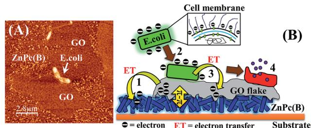
Fig. 10 (A) An AFM phase micrograph of *E. coli* cells adhered on ZnPc(B)–GO after 2 h incubation and a stand-by time period of 1 h under ambient conditions. (B) Schematic diagram illustrating the proposed mechanism for the interaction between the *E. coli* cells and ZnPc(B)–GO.
