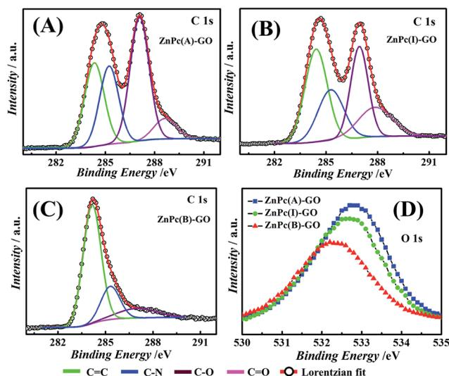
Fig. 5 Lorentzian deconvoluted peaks of the XPS spectra for (A) the C peak of ZnPc(A)-GO, (B) the C peak of ZnPc(I)-GO, (C) the C peak of ZnPc(B)-GO and (D) the O peaks of ZnPc(A)-GO, ZnPc(I)-GO and ZnPc(B)-GO. The symbols 'C' and 'O' represent elemental carbon and oxygen, respectively.
