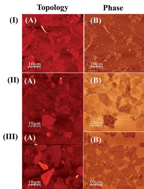
Fig. 4 AFM topographical and phase contrast images for the ZnPc-GO composites at various temperatures. The surface topography images (I(A)), (II(A)) and (III(A)) correspond to ZnPc(A)-GO, ZnPc(I)-GO and ZnPc(B)-GO, respectively. The phase contrast images (I(B)), (II(B)) and (III(B)) correspond to ZnPc(A)-GO, ZnPc(I)-GO and ZnPc(B)-GO, respectively.
