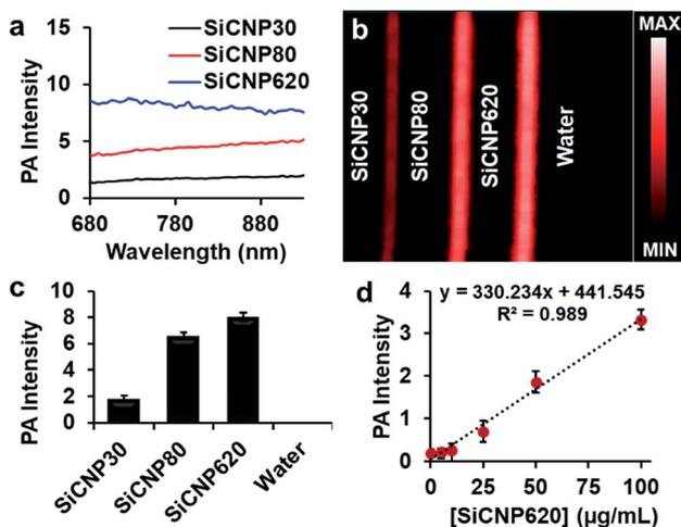
**Fig. 3** Photoacoustic properties of SiCNPs. (a) Photoacoustic spectra, (b) photoacoustic image and (c) the corresponding quantification of the photoacoustic intensity at 725 nm. (d) Photoacoustic signal of SiCNP620 was linearly dependent on the particle concentration. The limit of detection of SiCNP620 was found to be  $10 \mu\text{g mL}^{-1}$ . Error bars are standard deviations of 5 regions of interest.
