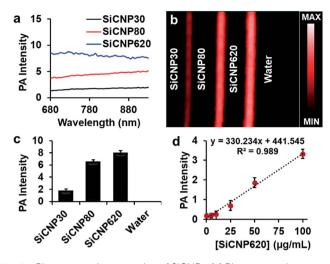
Fig. 3 Photoacoustic properties of SiCNPs. (a) Photoacoustic spectra, (b) photoacoustic image and (c) the corresponding quantification of the photoacoustic intensity at 725 nm. (d) Photoacoustic signal of SiCNP620 was linearly dependent on the particle concentration. The limit of detection of SiCNP620 was found to be 10  $\mu$ g mL<sup>-1</sup>. Error bars are standard deviations of 5 regions of interest.
