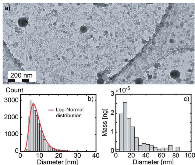
**Fig. 2** (a) Large field image ( $\times 20k$ ) of Gd<sub>2</sub>O<sub>3</sub> nanoparticles. (b) Size distribution of 19 310 nanoparticles deduced from 3 large field images (see Fig. S4 in ESI†) including image (a). The red curve corresponds to a log-normal distribution fit (median size = 8.0 nm, standard deviation = 3.6 nm). (c) Corresponding mass distribution of the nanoparticles (median size = 19.7 nm).
