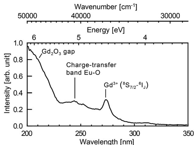
Fig. 5 Excitation spectrum of the nanoparticles synthesised in a solution of  $10^{-3}$  mol  $\text{L}^{-1}$  of europium salt. Emission at 625 nm integrated over 32 nm (FWHM of the spectral resolution). The spectral resolution of the excitation spectrum is 4 nm.
