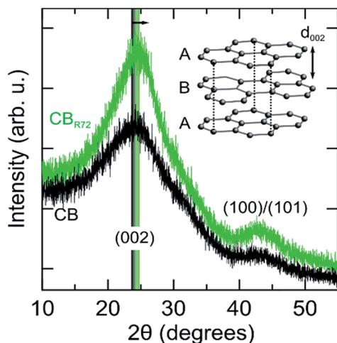
Fig. 6 XRD patterns of pristine (CB) and remotely photo-oxidized ( $CB_{R72}$ ) carbon black. The inset shows the graphene sheet-like stacking giving rise to the (002) Bragg diffraction peak, which is shifted to higher scattering angles (smaller inter-plane spacing) following photo-oxidation (arrow).
