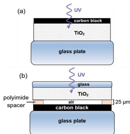
Fig. 2 Configuration of CB and TiO<sub>2</sub> layers. (a) Contact photocatalysis. (b) Remote photocatalysis experiments.
