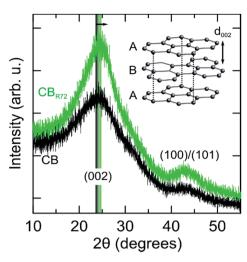
Fig. 6 XRD patterns of pristine (CB) and remotely photo-oxidized (CB $_{\rm R72}$ ) carbon black. The inset shows the graphene sheet-like stacking giving rise to the (002) Bragg diffraction peak, which is shifted to higher scattering angles (smaller inter-plane spacing) following photo-oxidation (arrow).
