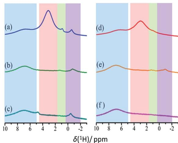
Fig. 3 Magic angle spinning <sup>1</sup>H NMR of (a) CB<sub>R72</sub>, (b) CB<sub>700</sub> and (c) pristine CB, and their respective dried versions (d), (e) and (f) at a spinning frequency of 40 kHz and at a static magnetic field of 11.74 T.
