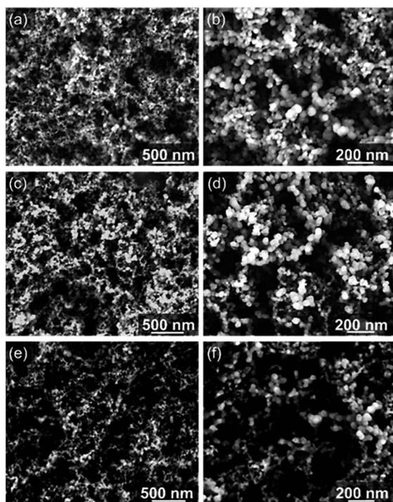
Fig. 7 HR SEM images. (a and b) Pristine CB. (c and d)  $CB_{R72}$ . (e and f)  $CB_{C72}$ . Both contact and remote experiments were performed simultaneously in the same reactor at 150 °C for 72 h with gas mixture 1.
