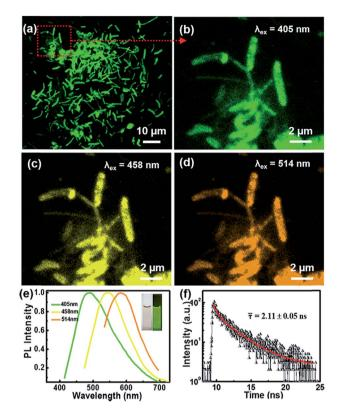
Fig. 3 (a) LCFM image of the full view of CNBs ( $\lambda_{\rm ex}=405$  nm). The enlarged LCFM images of CNBs were obtained under excitation at (b) 405 nm, (c) 458 nm and (d) 514 nm. (e) PL emission spectra of CNB aqueous solution. Inset: photos of the aqueous solution under sunlight and a UV lamp (365 nm). (f) PL decay lifetime spectrum and fitting curve (red line) of CNBs ( $\lambda_{\rm ex}=405$  nm).
