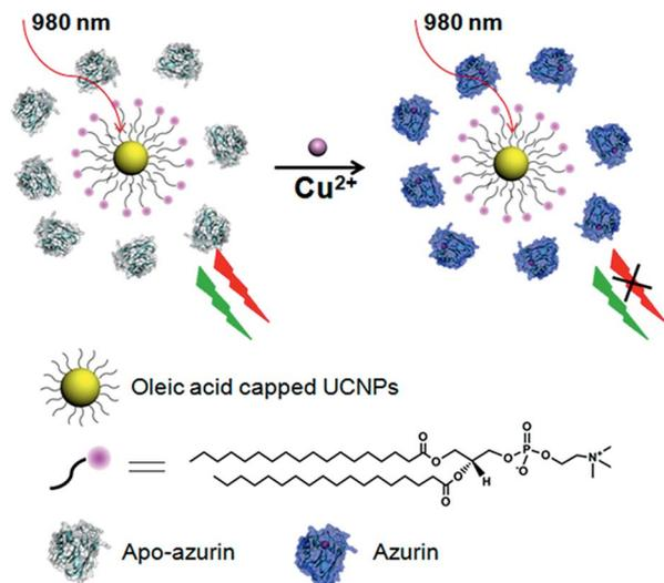
Fig. 1 Schematic illustration of the ratiometric upconversion luminescence sensing of  $\text{Cu}^{2+}$  based on an azurin-UCNP biosensor.
