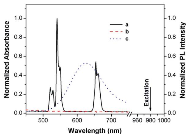
Fig. 2 UCL spectrum of DSPC-coated  $\text{NaYF}_4:20\%\text{Yb},2\%\text{Er}$  (DSPC-UCNP) under excitation from a 980 nm laser (a), and UV-vis spectra of the protein apo-azurin in the absence (b) and presence of  $\text{Cu}^{2+}$  (c).
