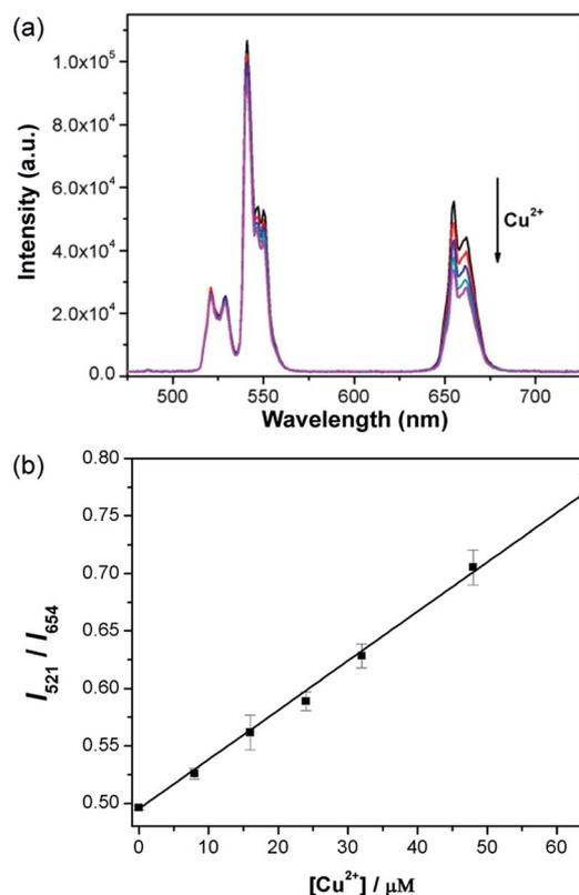
Fig. 5 (a) UCL spectra of the apo-azurin-UCNP system (under excitation from a 980 nm laser) in the presence of varying concentrations of Cu<sup>2+</sup> ions; (b) the ratio (I<sub>521</sub>/I<sub>654</sub>) of UCL intensities of the sensor system at 521 and 654 nm as a function of Cu<sup>2+</sup> concentration.
