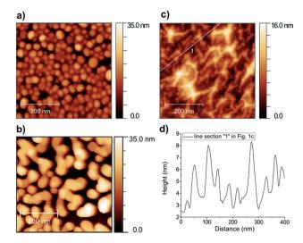
Fig. 1 Tapping mode AFM images of Au NPs obtained from annealing (a) 5 nm gold layer on  $SiO_2$ , (b) 10 nm gold layer on  $SiO_2$ . (c) Au NPs as in (a), but covered with graphene. (d) Height profile along the line section "1" in (c).
