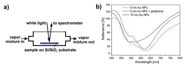
Fig. 2 (a) Schematic drawing of the aluminium cell used in the vapour sensing measurements. (b) Optical reflectance spectra of Au NPs and the annealed graphene/"5 nm" Au NPs samples measured in air.
