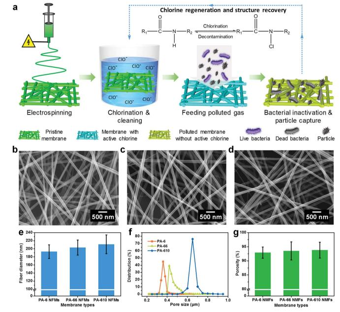
Fig. 1 (a) Schematic illustration of the design process of the versatile NFMs with rechargeable biocidal capacity and renewable air filtration performance. SEM images of pristine (b) PA-6, (c) PA-66, and (d) PA-610 NFMs. (e) Fiber diameter, (f) pore size, and (g) porosity of various PA membranes.
