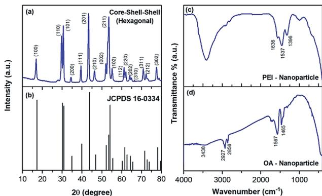
Fig. 2 (a) The powder X-ray diffraction pattern of  $\text{NaYF}_4\cdot\text{Yb}^{3+}/\text{Tm}^{3+}@/\text{NaYF}_4\cdot\text{Yb}^{3+}@/\text{NaYF}_4\cdot\text{Yb}^{3+}/\text{Nd}^{3+}$  nanoparticles. (b) The standard JCPDS data corresponding to file number 16-0334; the FTIR spectra of (c) poly(ethylenimine) coated (d) oleic acid coated upconverting nanoparticles (core-shell-shell).
