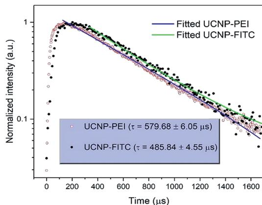
Fig. 5 Comparison of transients and fitting curves for the  ${}^1\text{G}_4 \rightarrow {}^3\text{H}_6$  transition (474 nm) of  $\text{Tm}^{3+}$  in PEI-coated UCNPs and FITC-conjugated UCNP upon excitation at 808 nm.
