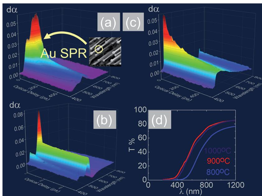
**Fig. 9** Ultrafast, differential transient absorption  $d\alpha$  versus optical delay  $\tau$  (ps) and probe wavelength  $\lambda$  (nm) through the Sb:SnO<sub>2</sub> NWs grown on r-Al<sub>2</sub>O<sub>3</sub> at (a) 800 °C, (b) 900 °C and (c) 1000 °C; (d) steady state transmission of light through the Sb:SnO<sub>2</sub> NWs grown on r-Al<sub>2</sub>O<sub>3</sub> at different temperatures.
