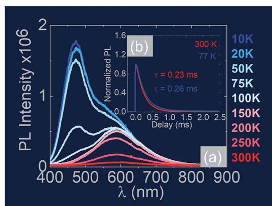
Fig. 10 (a) Temperature dependence of the PL obtained from the  $\text{Sb}:\text{SnO}_2$  NWs grown on  $r\text{-Al}_2\text{O}_3$  at  $800^\circ\text{C}$  (b) time resolved PL taken at  $\lambda = 600\text{ nm}$  for  $300\text{ K}$  and  $77\text{ K}$  along with the corresponding lifetimes.
