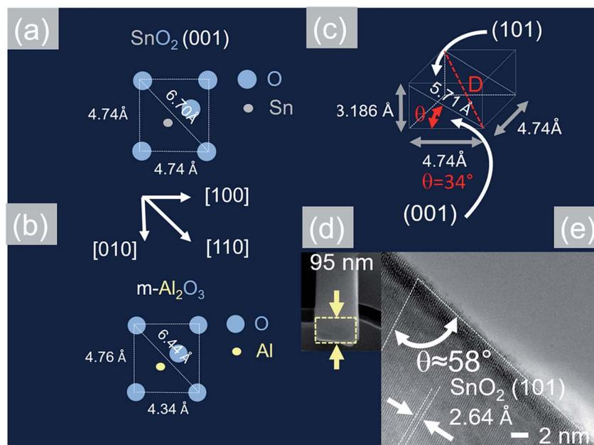
Fig. 5 (a) Two dimensional lattice of the SnO<sub>2</sub> (001) that is grown in an epitaxial way on (b) oxygen terminated m-Al<sub>2</sub>O<sub>3</sub> (c) crystal structure of tetragonal rutile SnO<sub>2</sub> (d) TEM and (e) HRTEM images of a Sb:SnO<sub>2</sub> NW after removing it from the m-Al<sub>2</sub>O<sub>3</sub>.
