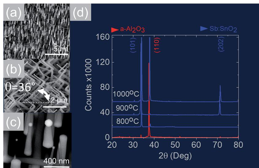
**Fig. 4** (a)–(c) SEM images of the Sb:SnO<sub>2</sub> NWs obtained at 800 °C on a-Al<sub>2</sub>O<sub>3</sub> (d) XRD of a-Al<sub>2</sub>O<sub>3</sub> (red) and Sb:SnO<sub>2</sub> NWs (blue) grown on a-Al<sub>2</sub>O<sub>3</sub> at 800 °C, 900 °C and 1000 °C.
