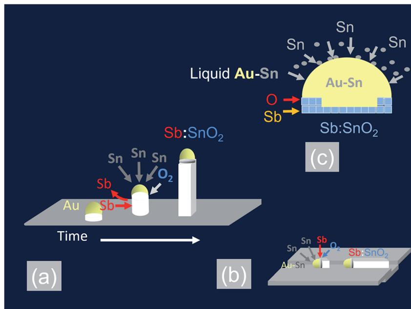
Fig. 1 Schematic representation of the VLS growth mechanism of Sb:SnO<sub>2</sub> NWs (a) bottom-up growth (b) lateral growth along a step or groove (c) Sb donor impurity incorporation mechanism.
