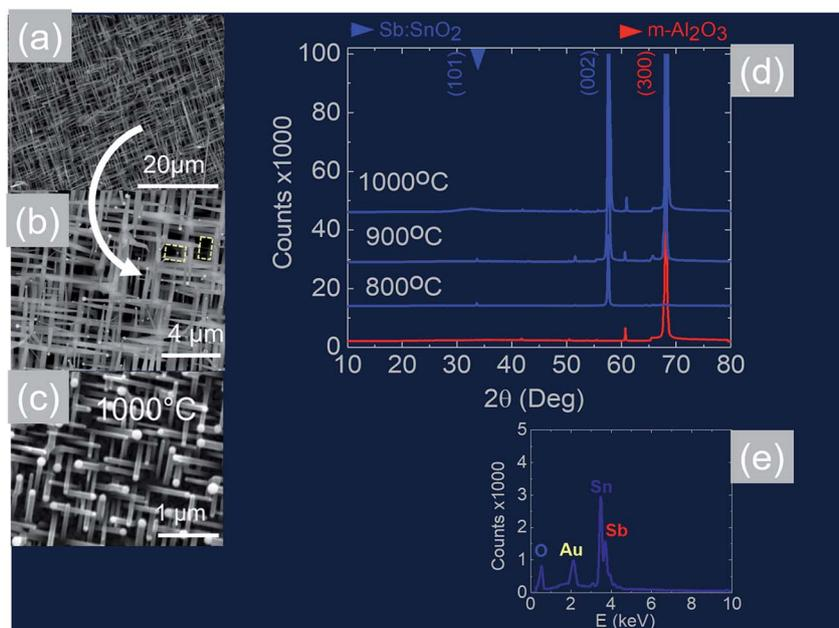
Fig. 2 SEM images of the Sb:SnO<sub>2</sub> NWs obtained at (a), (b) 800 °C and (c) 1000 °C on m-Al<sub>2</sub>O<sub>3</sub> (d) XRD of m-Al<sub>2</sub>O<sub>3</sub> (red) and Sb:SnO<sub>2</sub> NWs (blue) grown on m-Al<sub>2</sub>O<sub>3</sub> at 800 °C, 900 °C and 1000 °C (e) EDX of the Sb:SnO<sub>2</sub> NWs.
