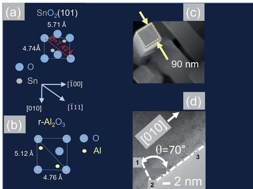
Fig. 6 (a) Two dimensional surface lattice of  $\text{SnO}_2(101)$  which grows on (b) oxygen terminated surface of  $r\text{-Al}_2\text{O}_3$  (c) TEM image of  $\text{Sb}:\text{SnO}_2$  NWs after removing from  $r\text{-Al}_2\text{O}_3$  (d) HRTEM image of the  $\text{Sb}:\text{SnO}_2$  NWs showing the (010) lattice planes.
