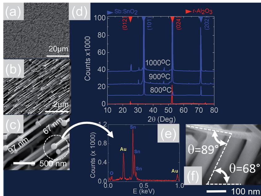
**Fig. 3** (a)–(c) SEM images of the Sb:SnO<sub>2</sub> NWs obtained at 800 °C on r-Al<sub>2</sub>O<sub>3</sub> (d) XRD of r-Al<sub>2</sub>O<sub>3</sub> and Sb:SnO<sub>2</sub> NWs grown at 800 °C, 900 °C and 1000 °C (e) EDX of an Au:Sn particle on the end of a Sb:SnO<sub>2</sub> NW (f) side view showing that the first segment of the Sb:SnO<sub>2</sub> NWs grows at  $\theta = 68^\circ$  and the second segment at  $\theta = 89^\circ$  with respect to the first.
