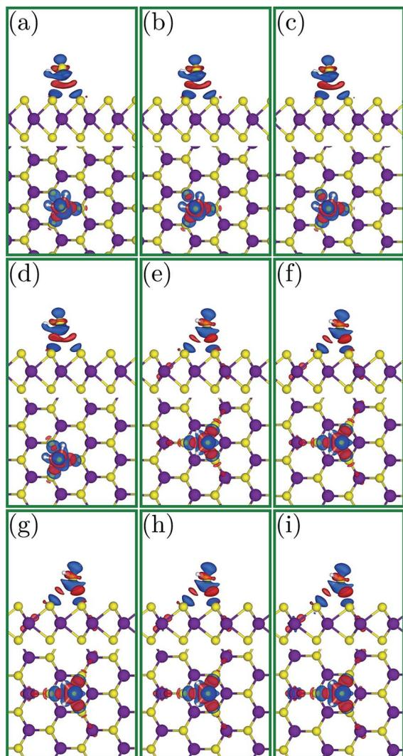
Fig. 6 Top (upper) and side (lower) views of the charge density difference ( $\Delta\rho$ ) for the least-energy configurations between the  $\text{H}_2\text{S}$  molecule and SL-MoS<sub>2</sub>. (a)–(i) correspond to  $-8\%$  to  $+8\%$  biaxial strains with intervals of  $2\%$ .
