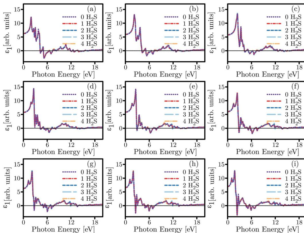
Fig. 9 The real ( $\epsilon_1$ ) part of the dielectric function for pristine and H<sub>2</sub>S adsorbed SL-MoS<sub>2</sub> for (a) –8 percent to (h) +8 percent strained substrates with 2-percent intervals. Moreover, the influence of concentration is also shown.
