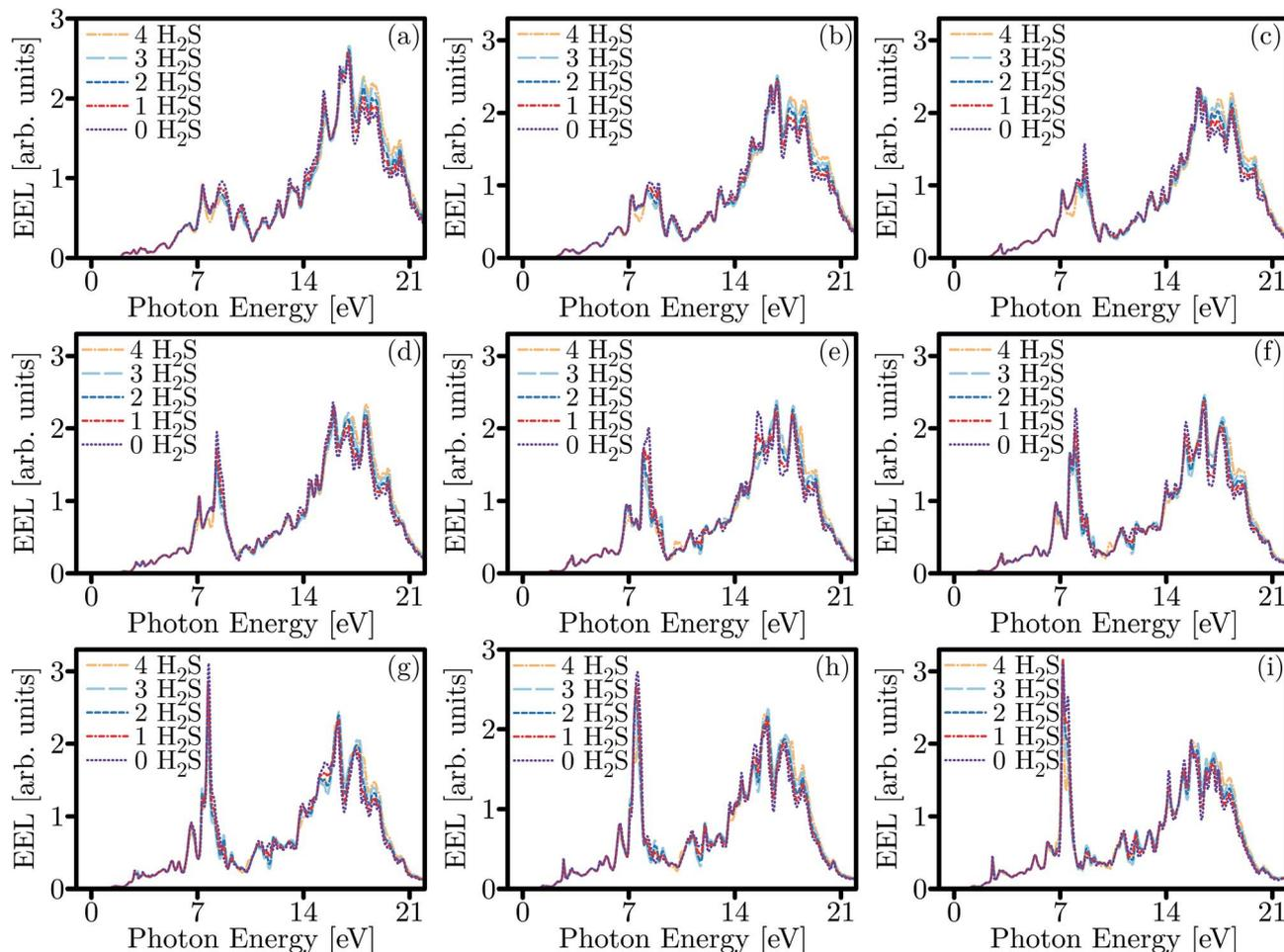
Fig. 11 Electron energy loss (EEL) spectra for the adsorption of up to four  $\text{H}_2\text{S}$  molecules in the supercell of SL-MoS<sub>2</sub> for in-plane light polarization under the application of biaxial strains from (a)  $-8\%$  to (h)  $+8\%$  with 2-percent intervals.
