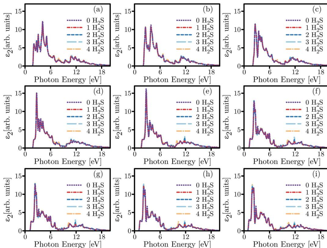
Fig. 10 The imaginary ( $\epsilon_2$ ) part of the dielectric function for pristine and  $\text{H}_2\text{S}$  adsorbed SL- $\text{MoS}_2$  for (a)  $-8$  percent to (h)  $+8$  percent strained substrates with 2-percent intervals. Moreover, the influence of concentration is also shown.
