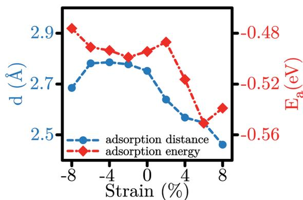
Fig. 4 Modulation of the adsorption distance ( $d$ ) and the adsorption energy ( $E_a$ ) for the H<sub>2</sub>S molecule in the most stable configurations for each value of strain.
