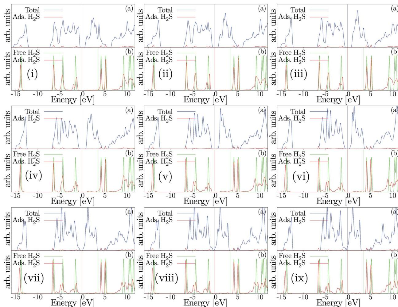
Fig. 8 Total density of states (DOS) (blue), DOS for the isolated H<sub>2</sub>S molecule (green), and DOS for the adsorbed H<sub>2</sub>S molecule (red) for both strained and unstrained conditions. (i) to (ix) represent –8% to 8% strained substrates with intervals of 2%. Vertical lines represent Fermi levels of their homochromatic graphs.
