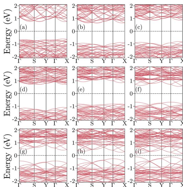
Fig. 7 Band structures for the adsorption of the  $\text{H}_2\text{S}$  molecule on (a)  $-8$  to (i)  $+8$  percent strained SL-MoS<sub>2</sub> substrates with 2 percent intervals.
