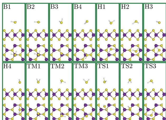
Fig. 2 Relaxed configurations of the H<sub>2</sub>S molecule above the unstrained SL-MoS<sub>2</sub> surface are shown. In each subsection, both the side view and the bird's eye view are shown. Purple (yellow) atoms represent molybdenum (sulfur).
