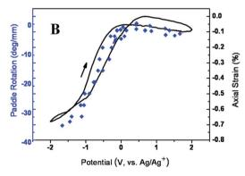
Fig. 13 Electrochemical torsional and tensile actuation for two-end-tethered, neat MWNT yarns half immersed in liquid electrolyte. Yarns were either prepared as S twist (A) or Z twist (B). Negative paddle rotations indicate rotation in the untwist direction and negative strains indicate length contraction. This figure has been reproduced from ref. 3 with permission from AAAS.
