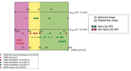
Fig. 5 VSSA distribution of the characterized powders and the corresponding  $d_{VSSA}$ .
