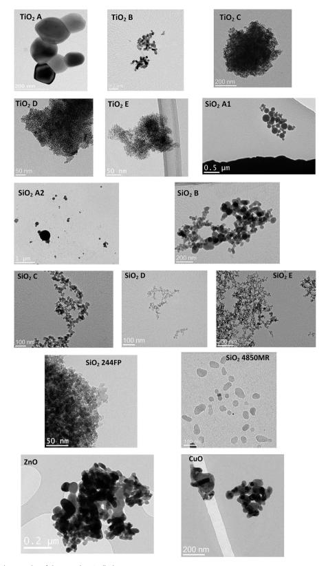
Fig. 4 Typical TEM micrographs of the powder studied.
