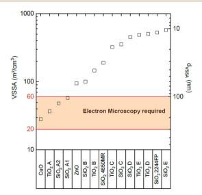
Fig. 3 VSSA distribution of the characterized powders and the corresponding  $d_{\rm VSSA}$  for a spherical particle shape assumption (shape factor D=3).
