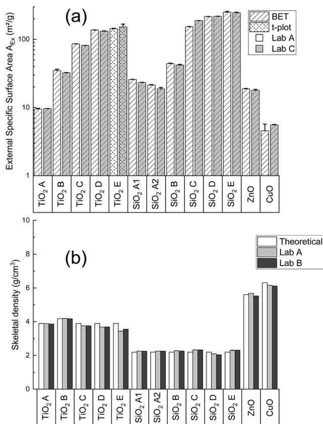
Fig. 2 (a) Comparison of the  $A_{\text{Ex}}$  obtained in Lab A and Lab C with N<sub>2</sub> adsorption measurements and (b) comparison of the experimental skeletal densities obtained in Lab A and Lab B with the theoretical material densities.
