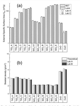
Fig. 2 (a) Comparison of the  $A_{\rm Ex}$  obtained in Lab A and Lab C with N<sub>2</sub> adsorption measurements and (b) comparison of the experimental skeletal densities obtained in Lab A and Lab B with the theoretical material densities.
