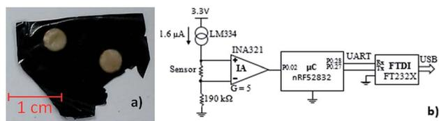
Fig. 8 (a) SF/CNT 1 wt% CNT content film with 4 gold electrodes (2 on the top and 2 on the bottom); (b) schematic of the test circuit, consisting in a current source and an instrumentation amplifier (IA).
