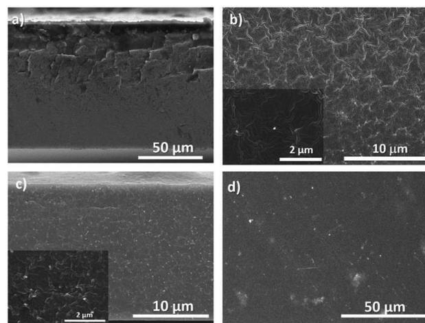
Fig. 2 SEM cross-sectional images of neat SF (a) and SF/CNT composites with 0.75 wt% CNTs (b) and 6 wt% CNTs (c) and the surface image of 6 wt% CNTs (d).
